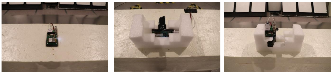
Photograph 1: EUT orientation during the test (X-, Y-, Z-orientation)
