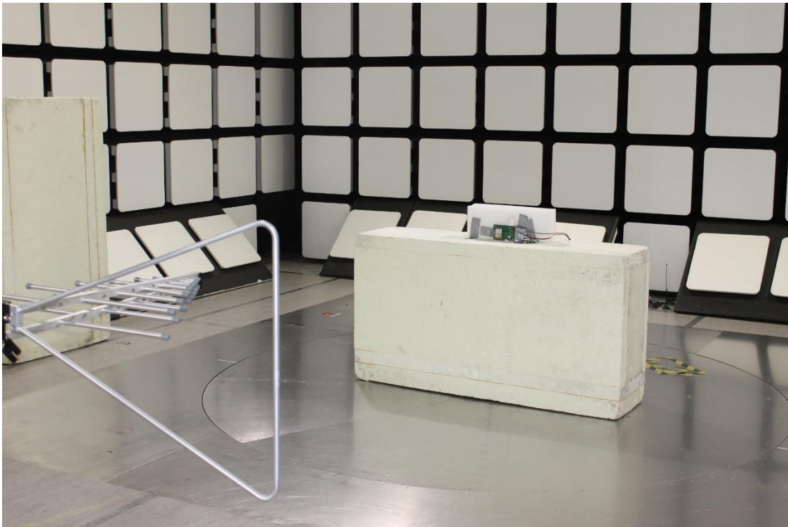
Photograph 5: Setup for spurious radiated emissions 30 - 1000 MHz
