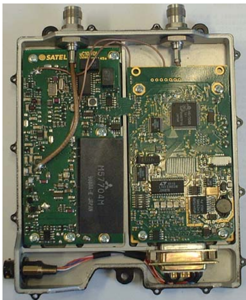
Picture 2. Inside of the Pi Research P192-S
