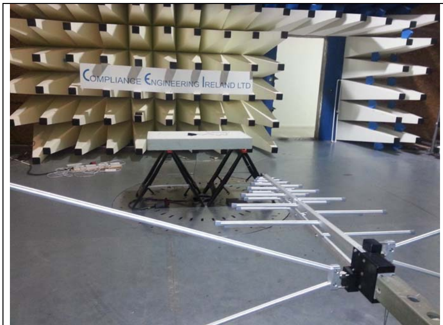
Fig 1 Test setup 30MHz -1GHz Rad Emission
