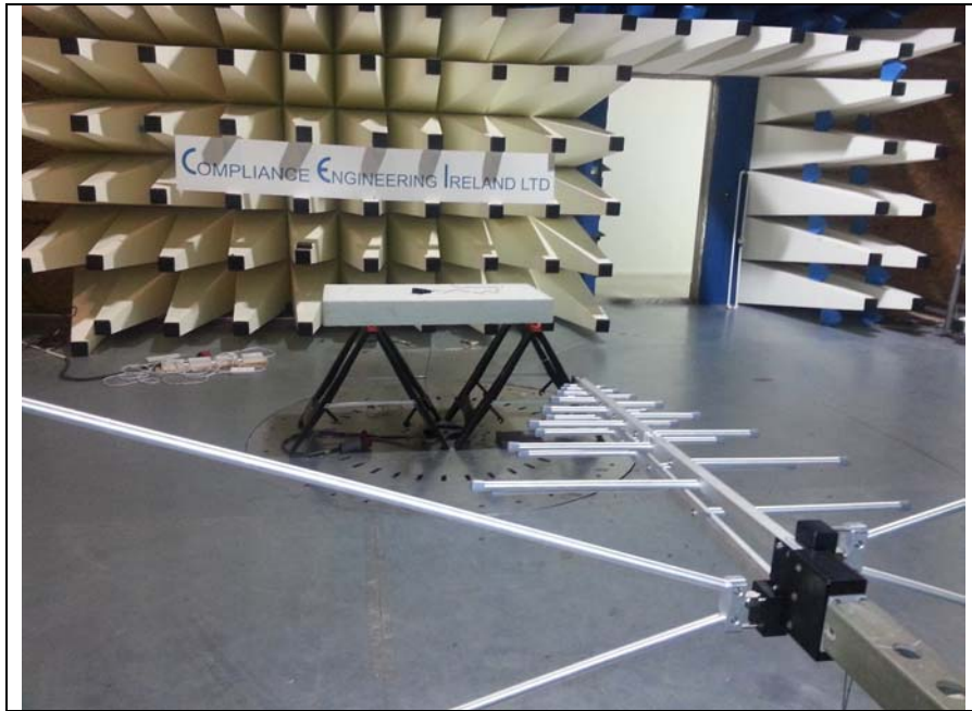
Fig 1 Test setup 30MHz -1GHz Rad Emission
