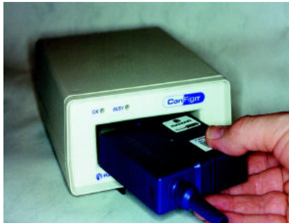
Figure 3 - A TransPondIT being configured in a ConFigIT
