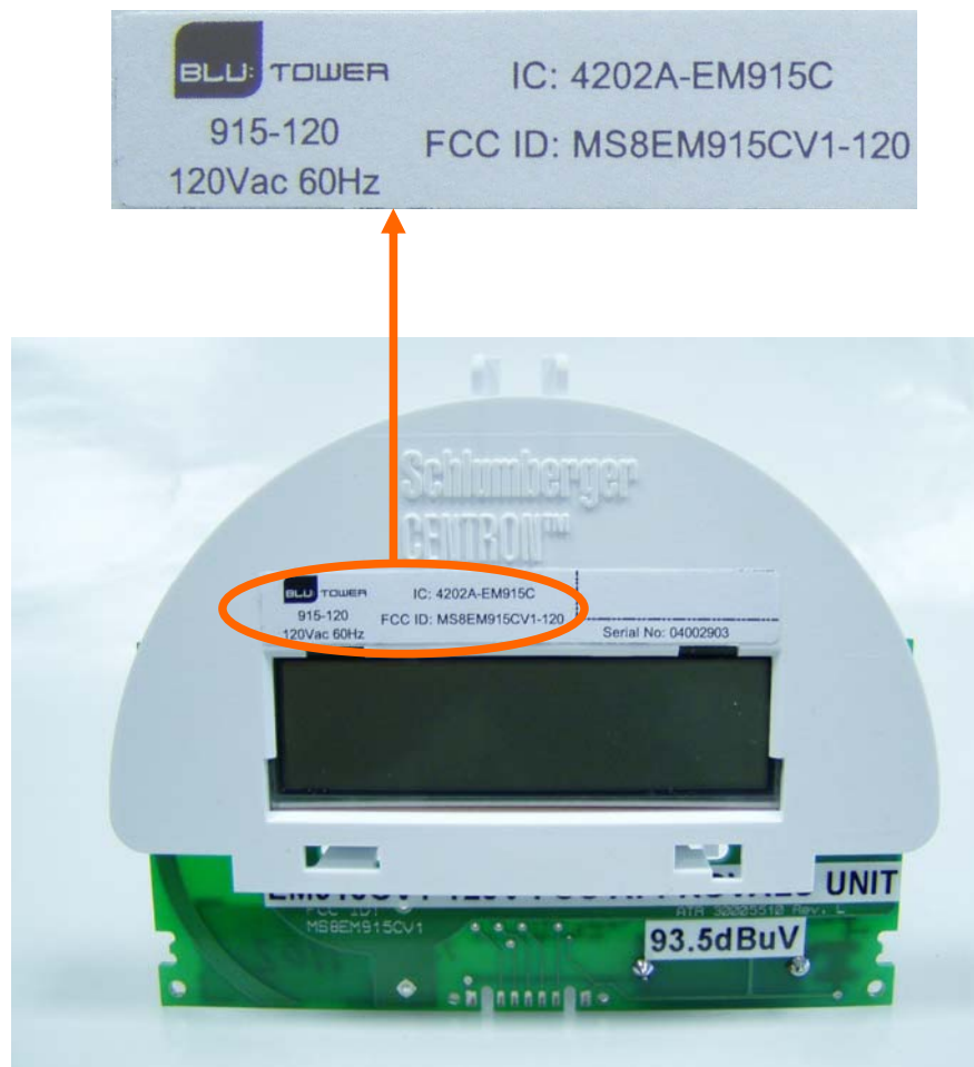
Figure 1: TransPondIT Centron 120V module (removed from meter): LCD front view
