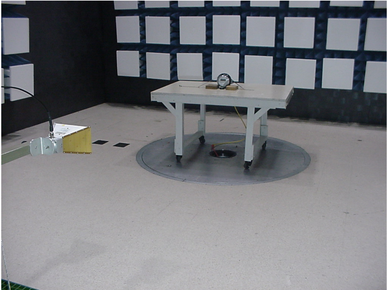
Figure 4 - Radiated Emissions Test Setup (Chamber - Front)
