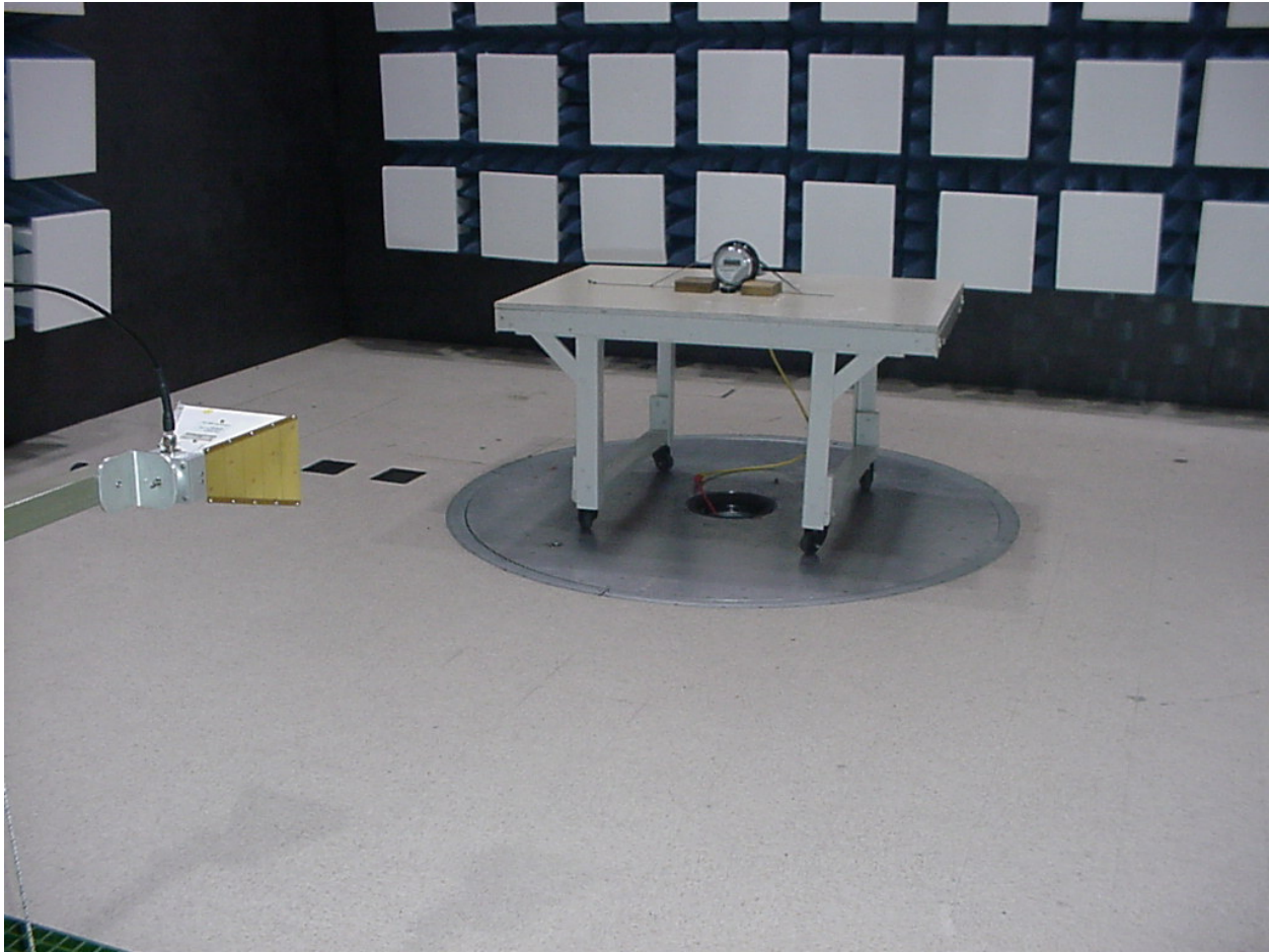
Figure 7 - Radiated Emissions Test Setup (Chamber - Front)
