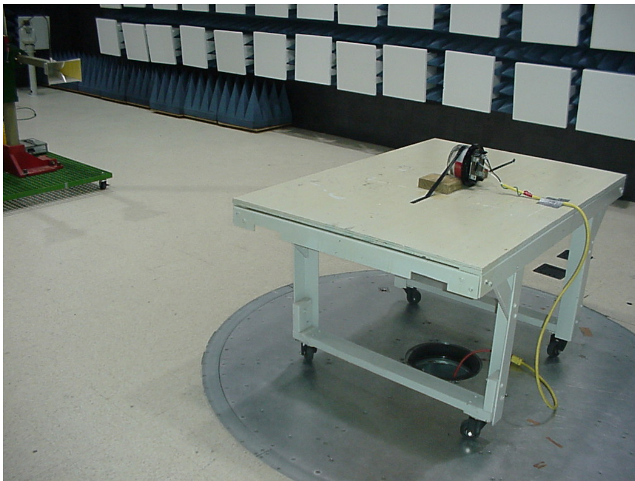
Figure 5 - Radiated Emissions Test Setup (Chamber - Back)
