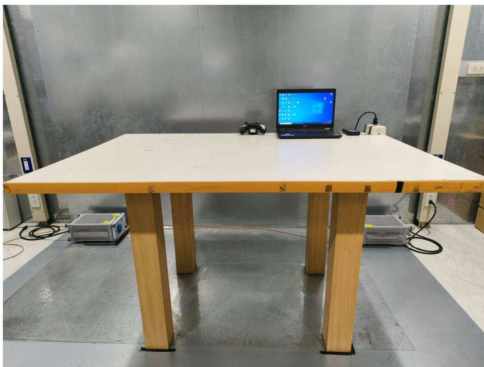
Back View of AC Power Line Conducted Emission Test
