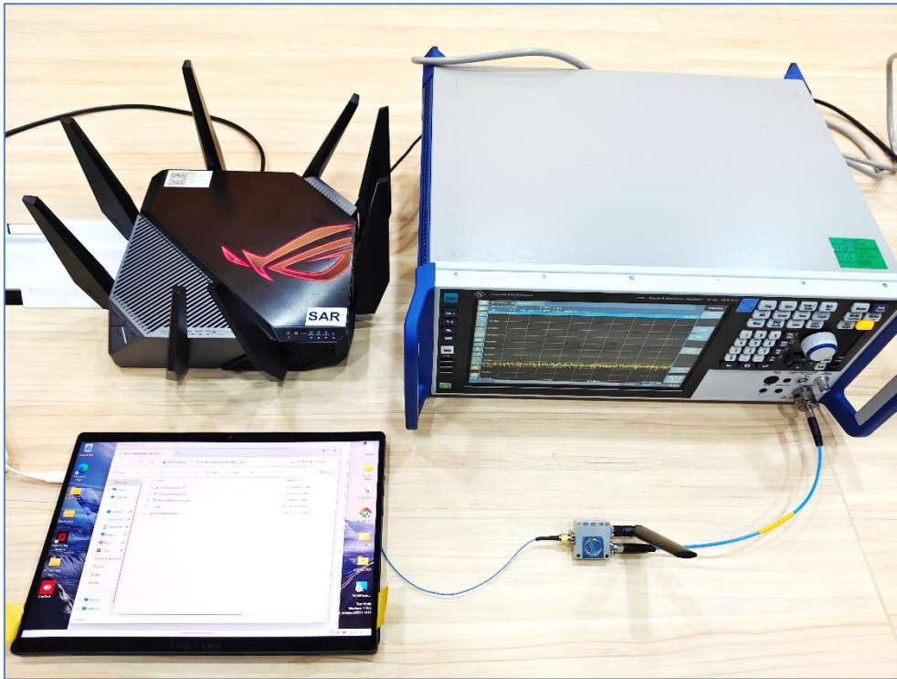
Setup for Conducted Power Testing (Test Scenario 1 and 4)
