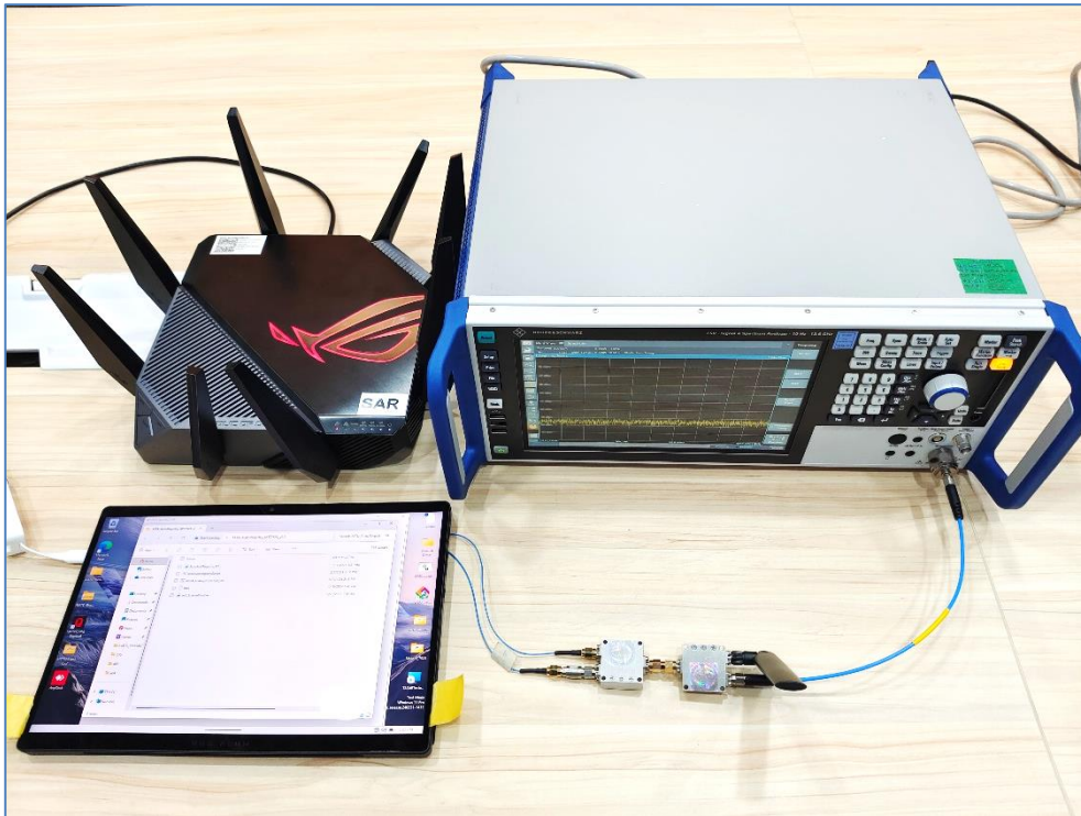
Setup for Conducted Power Testing (Test Scenario 3)
