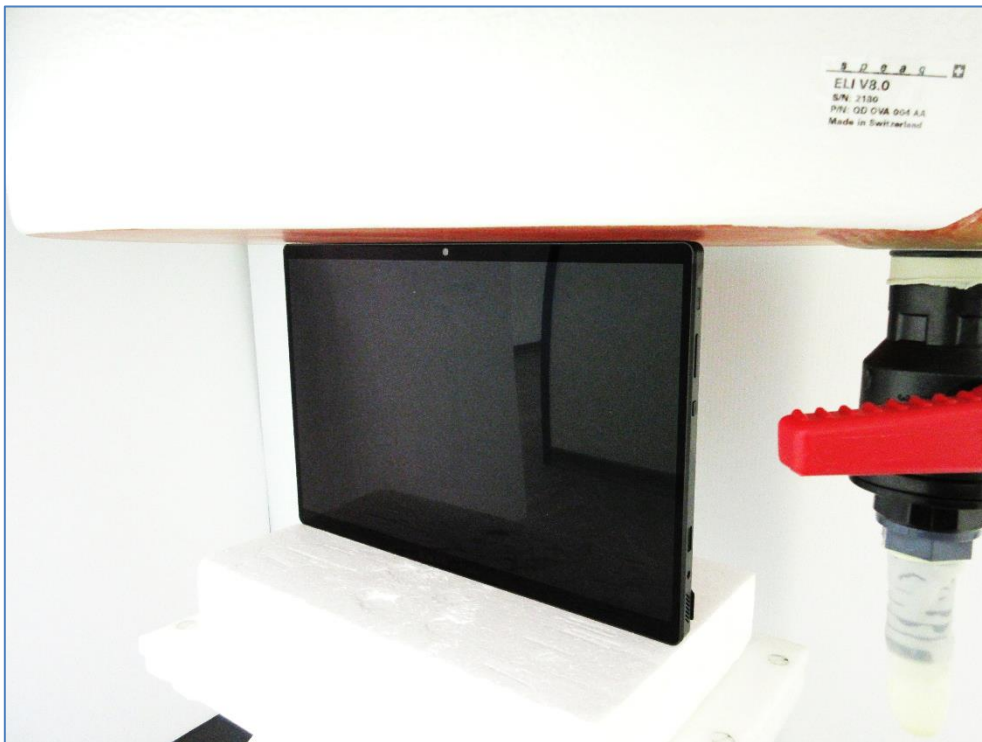
Setup for SAR Testing (Body, Tablet - Top Side at 0 mm)
