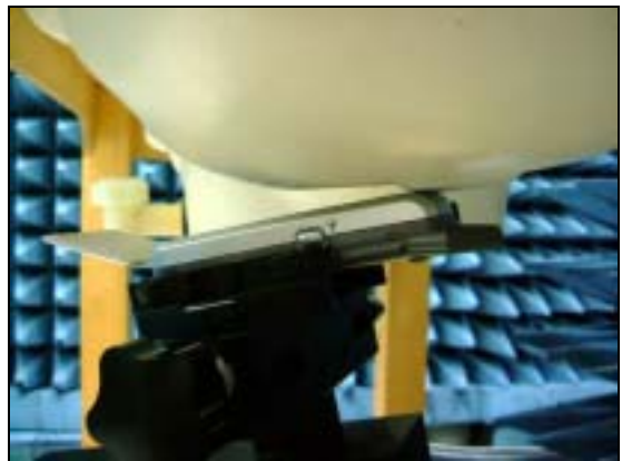
Figure 15. Right Head SAR Test Setup (Tilted)
