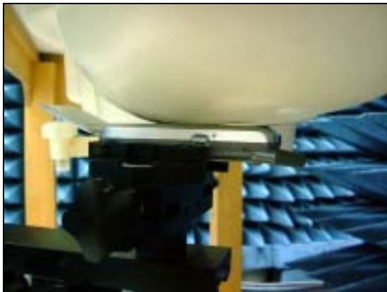
Figure 14. Right Head SAR Test Setup (Cheek)
