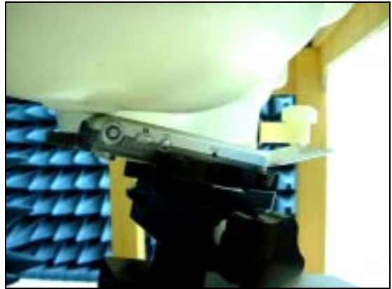
Figure 13. Left Head SAR Test Setup (Tilted)
