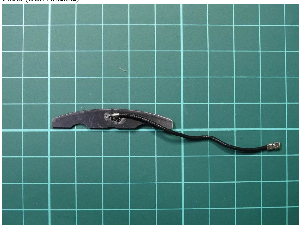
(30) EUT Photo (BLE Antenna)
