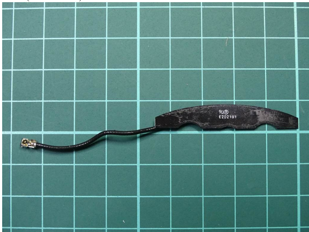
(31) EUT Photo (BLE Antenna)
