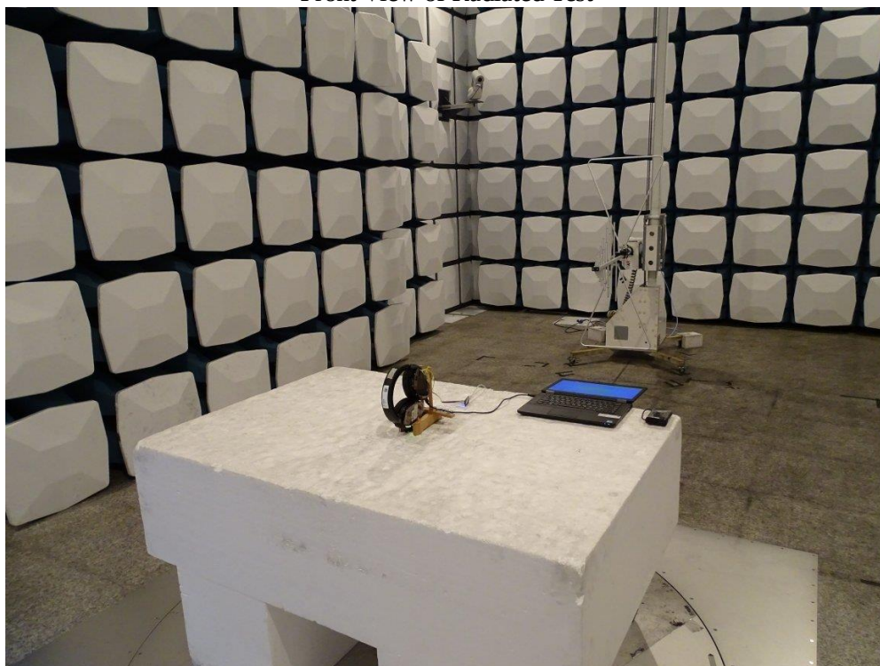
Front View of Radiated Test
