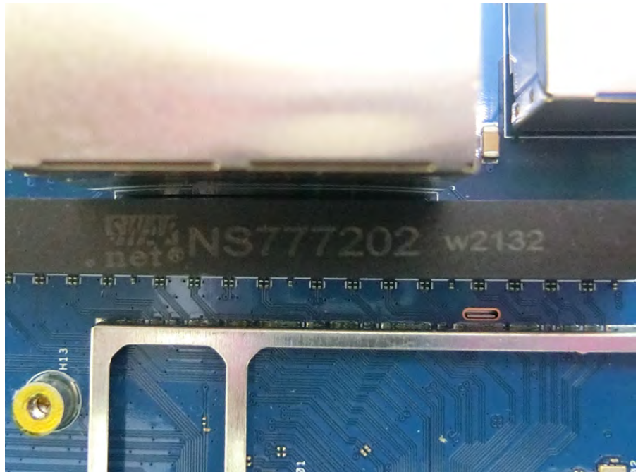
Transformer of 1Gbps LAN (Main Source)
