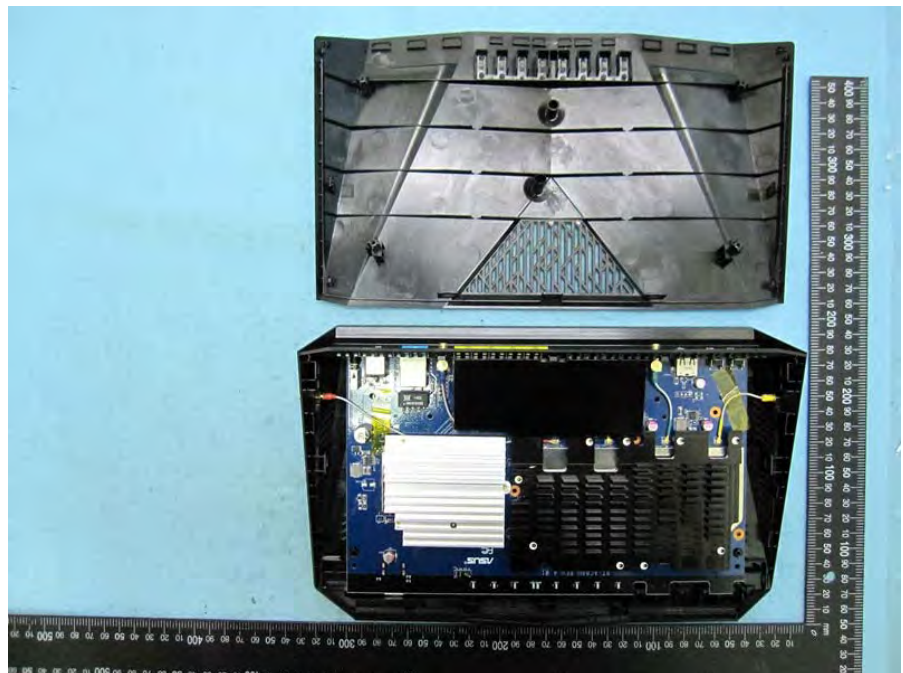
Black Heat sink (for model name: RT-AC3100)
