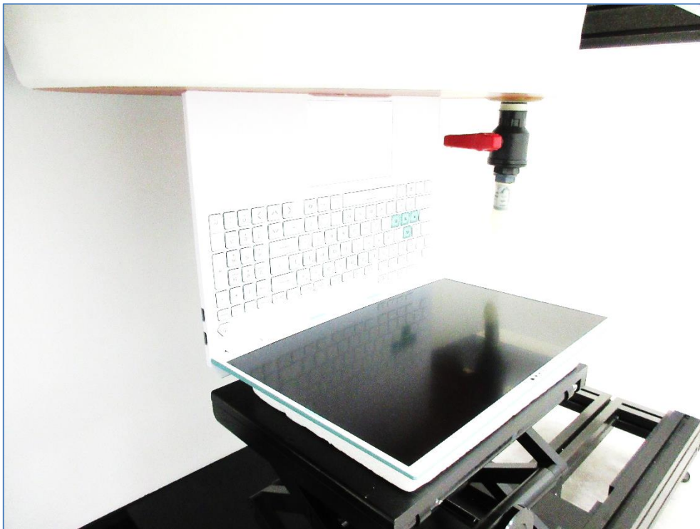
Setup for SAR Testing (Body, Front Edge of Laptop at 0 mm)
