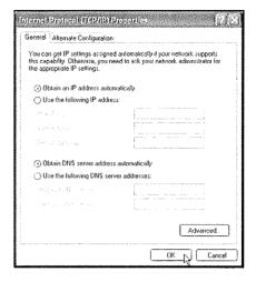
To set up the connection with a manually assigned IP address, the address of your PC and the wireless router must be within the same subnet:
