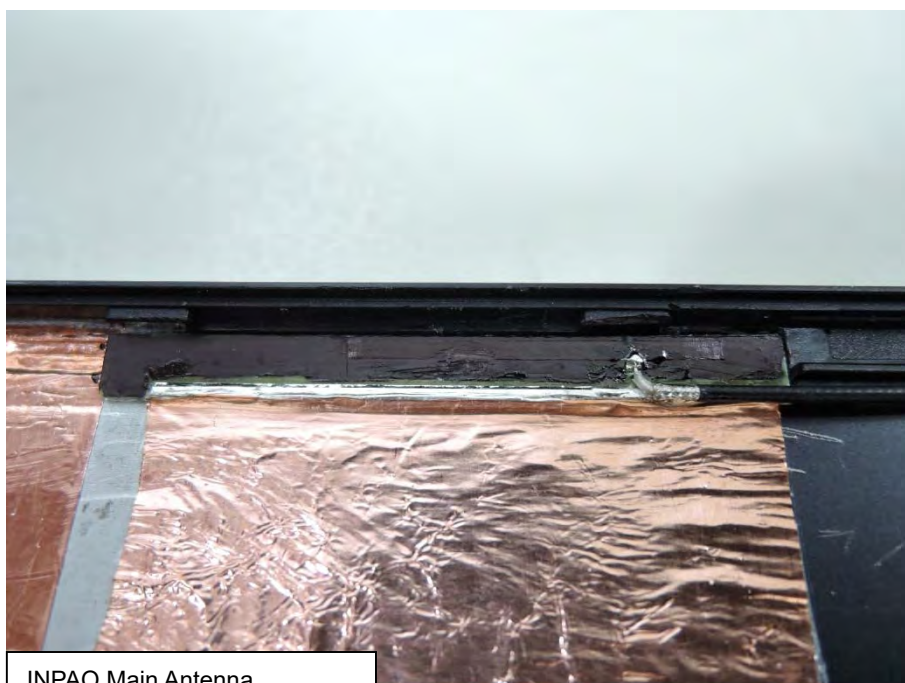
INPAQ Main Antenna Part No.: WA-P-LBLB-04-081
