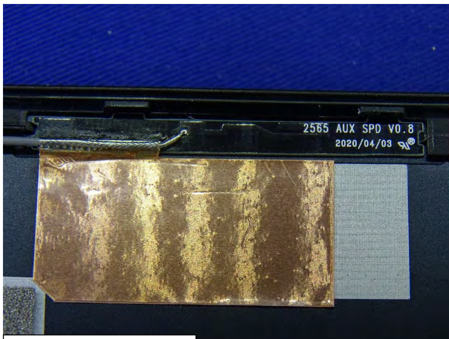
SPEED Aux Antenna Part No.: F-0G-XZ-0231-000-00
