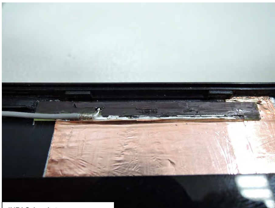
INPAQ Aux Antenna Part No.: WA-P-LBLB-04-081
