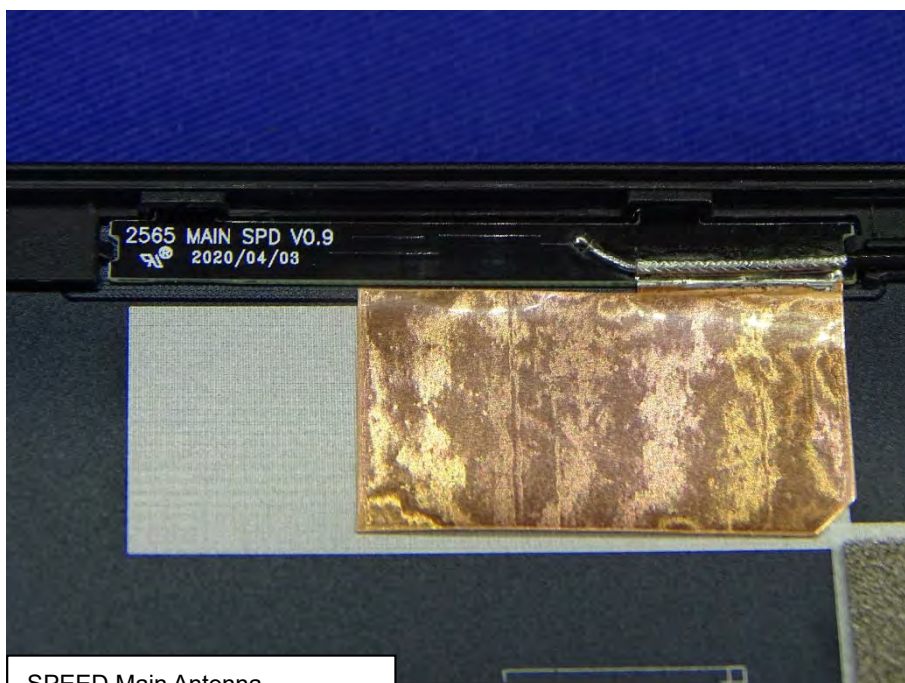
SPEED Main Antenna Part No.: F-0G-XZ-0231-000-00
