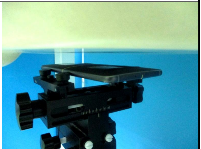
Rear Face of EUT with 1.5 cm Gap
