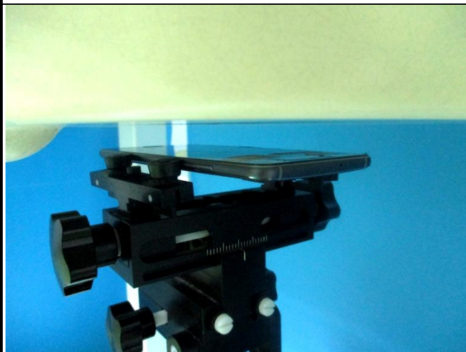
Front Face of EUT with 1.5 cm Gap
