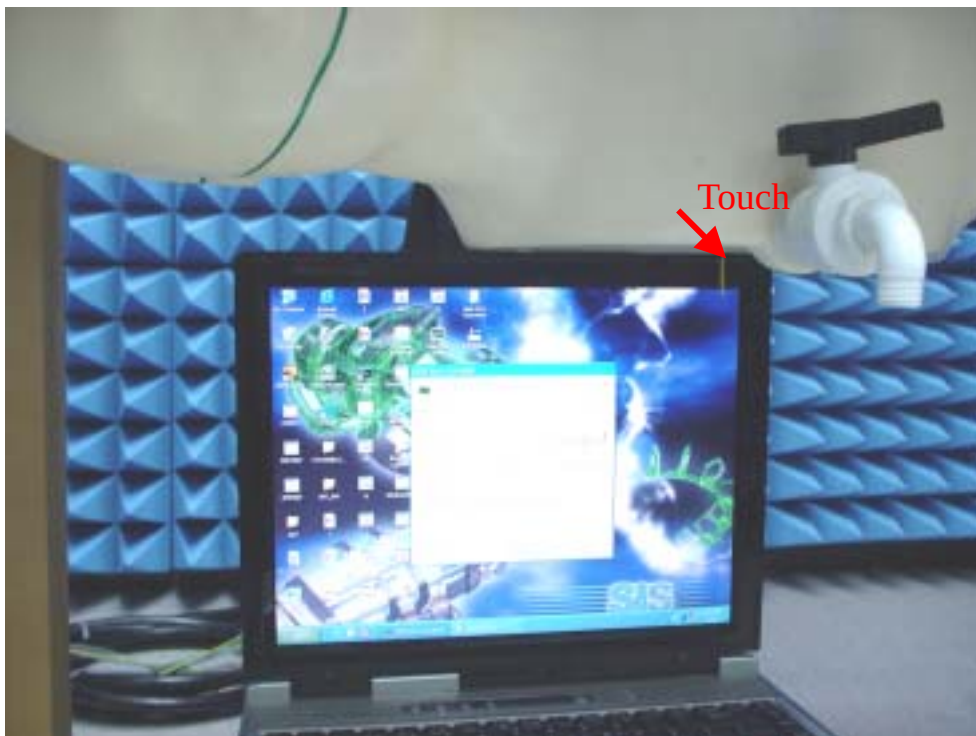
Fig.2 Photograph of the top of the LCD panel of Main Antenna contact to the flat Phantom; and at a distance of 0.0 cm from the base of the phantom.
