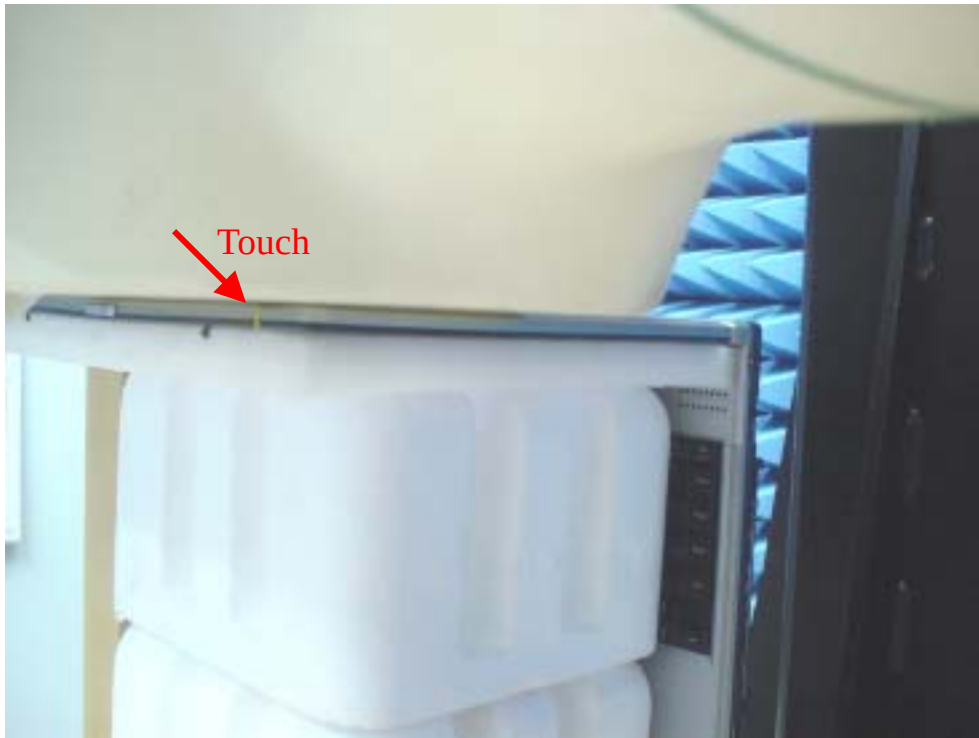
Fig.3 Photograph of the back of the LCD Panel of Right Antenna contact to the flat phantom; and at a distance of 0.0 cm from the base of the phantom
