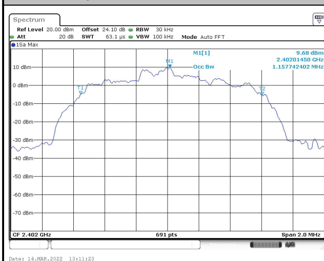
99% Occupied Bandwidth Plot on Channel 00
