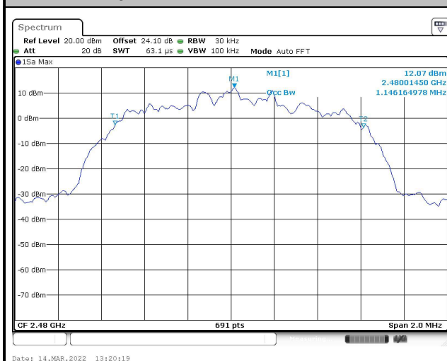
99% Occupied Bandwidth Plot on Channel 78
