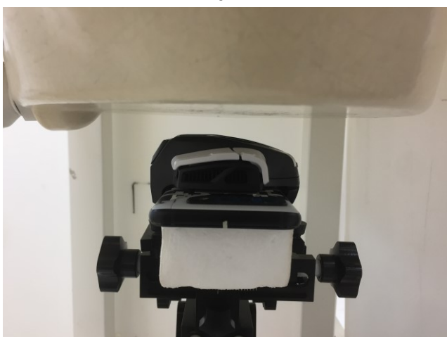
Back with AeroActive cooler, Test Separation 15 mm
