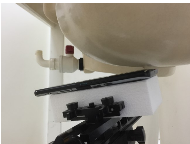
Left Tilted, Test Separation 0 mm
