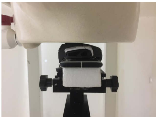
Back with AeroActive cooler, Test Separation 0 mm
