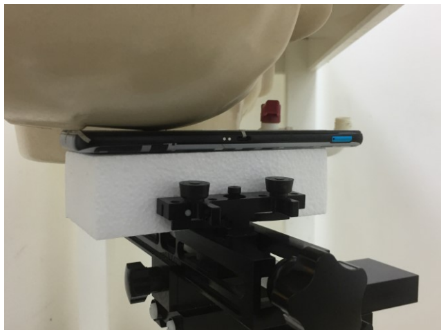
Right Cheek, Test Separation 0 mm
