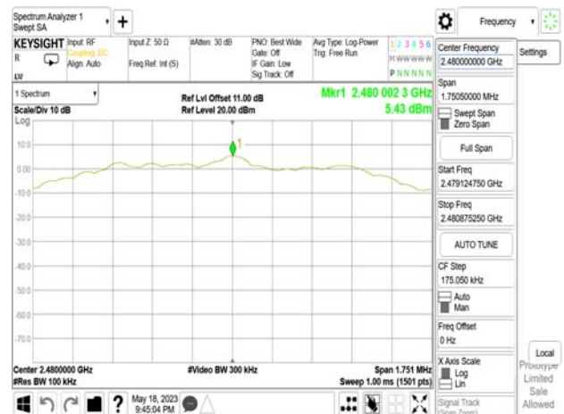
Reference Level_BLE 2M_HighCH39-2480MHz
