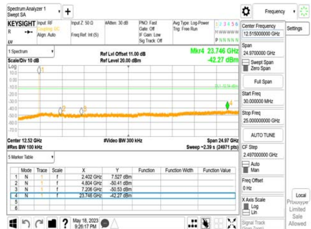
Spurious Emission_BLE 1M_MidCH20-2442MHz
