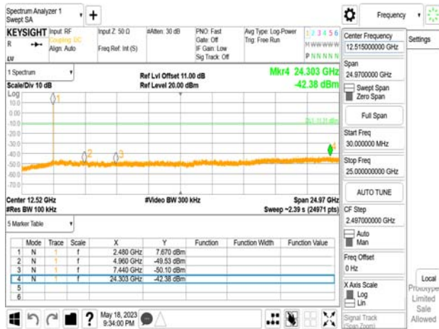
Spurious Emission_BLE 2M_LowCH00-2402MHz
