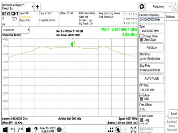
Reference Level_BLE 1M_HighCH39-2480MHz
