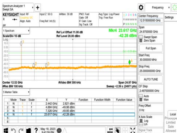
Spurious Emission_BLE 2M_MidCH20-2442MHz
