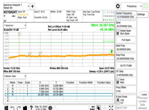
Spurious Emission_BLE 1M_MidCH20-2442MHz
