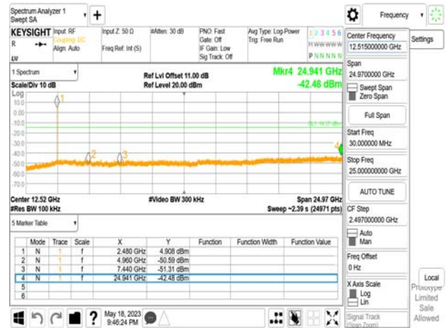
Spurious Emission_BLE 2M_HighCH39-2480MHz
