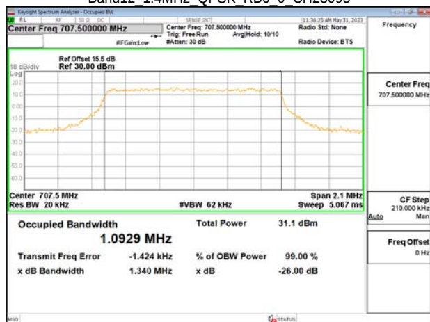
Band12 1.4MHz QPSK RB6 0 CH23173
