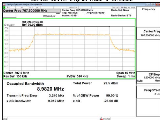
Band12 10MHz 64QAM RB50 0 CH23130
