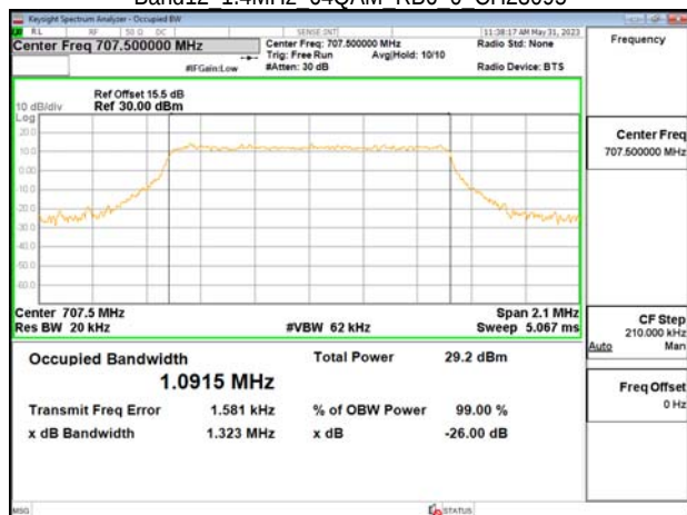
Band12 1.4MHz 64QAM RB6 0 CH23173
