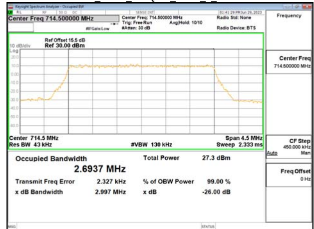
Band12 3MHz 256QAM RB15 0 CH23165
