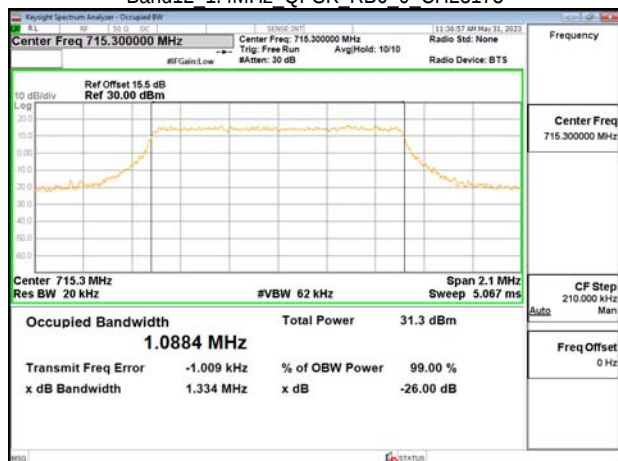
Band12 1.4MHz QPSK RB6 0 CH23173
