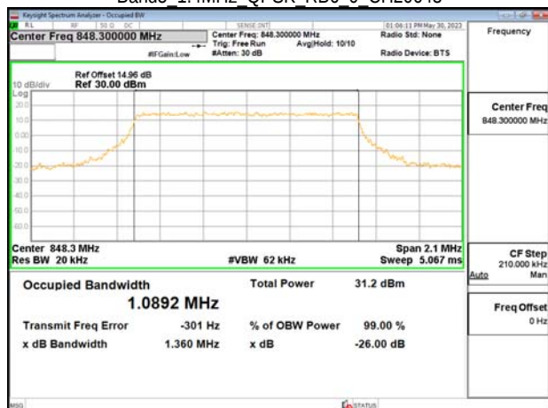
Band5 1.4MHz QPSK RB6 0 CH20643
