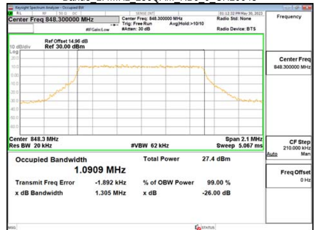
Band5 1.4MHz 256QAM RB6 0 CH20643
