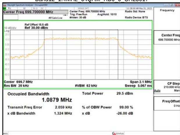
Band12 1.4MHz 64QAM RB6 0 CH23095
