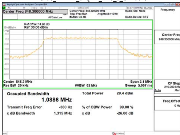
Band5 1.4MHz 64QAM RB6 0 CH20643
