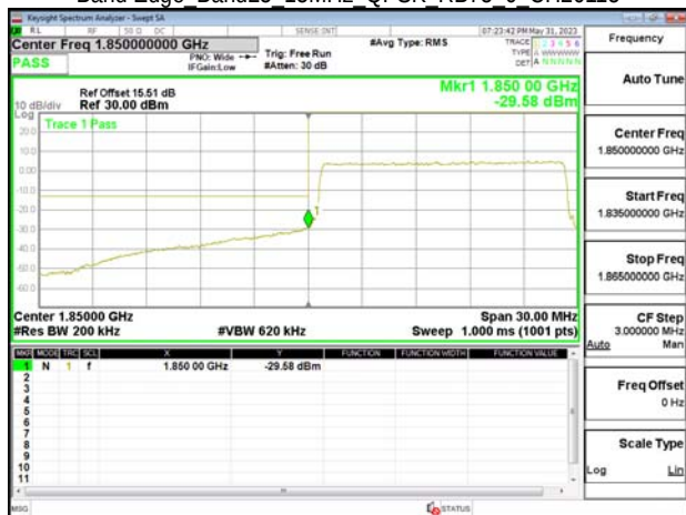
Band Edge Band25 15MHz QPSK RB75 0 CH26115
