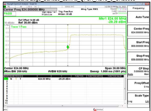
Band Edge Band26 15MHz QPSK RB75 0 CH26865
