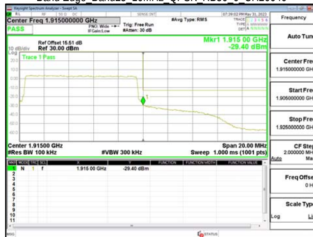
Band Edge Band25 10MHz QPSK RB50 0 CH26640
