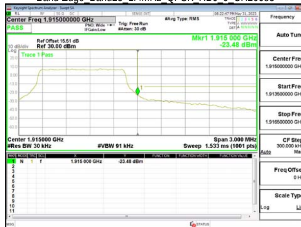
Band Edge Band25 1.4MHz QPSK RB6 0 CH26683
