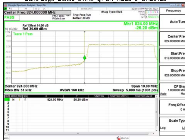
Band Edge Band5 5MHz QPSK RB25 0 CH20625
