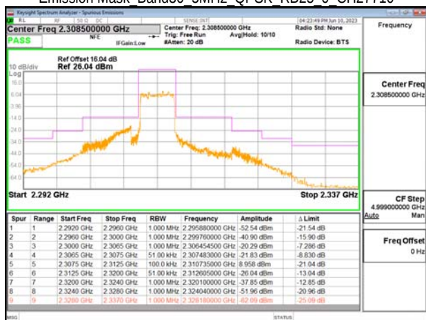
Emission Mask Band30 5MHz QPSK RB25 0 CH27710
