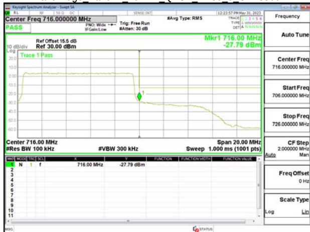
Band Edge Band25 1.4MHz QPSK RB1 0 CH26047
