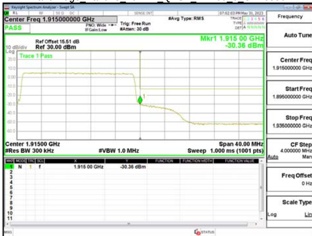
Emission Mask Band26-Part90s 1.4MHz QPSK RB1 0 CH26697
