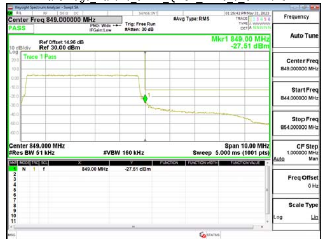
Band Edge Band26 10MHz QPSK RB1 0 CH26840
