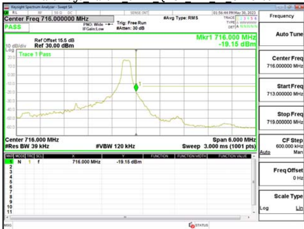
Band Edge Band12 3MHz QPSK RB15 0 CH23025
