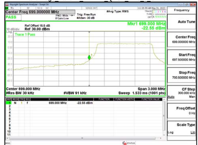
Band Edge Band12 1.4MHz QPSK RB6 0 CH23173
