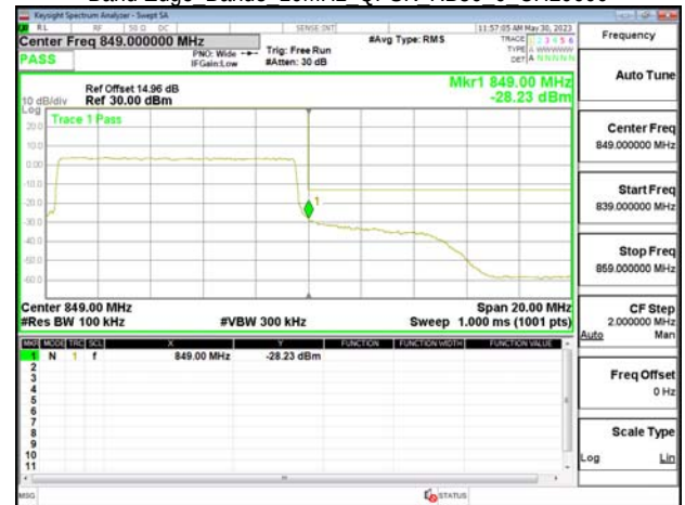
Emission Mask Band7 5MHz QPSK RB1 0 CH20775
