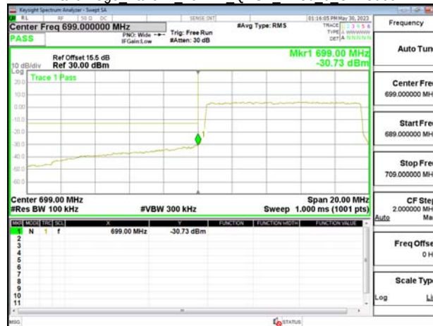
Band Edge Band12 10MHz QPSK RB50 0 CH23130
