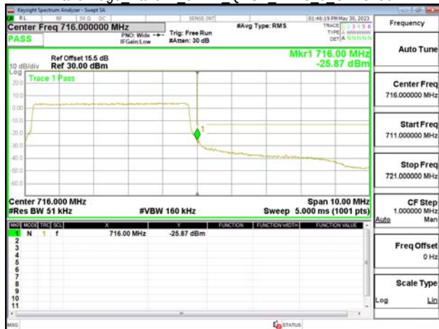
Band Edge Band12 10MHz QPSK RB1 0 CH23060
