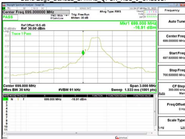
Band Edge Band12 1.4MHz QPSK RB1 0 CH23017
