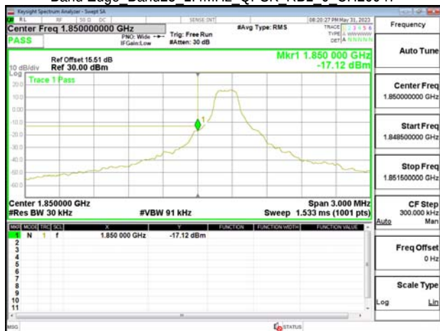
Band Edge Band25 1.4MHz QPSK RB1 0 CH26047
