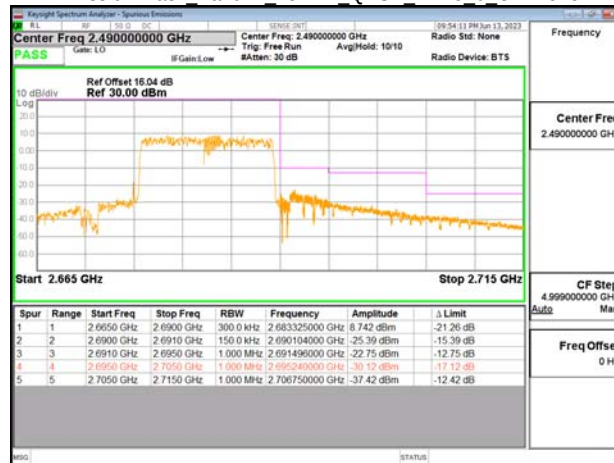
Emission Mask Band41 20MHz QPSK RB1 0 CH39750
