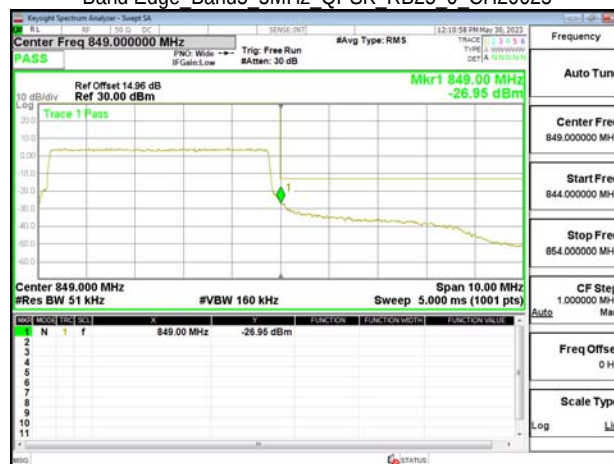
Band Edge Band5 5MHz QPSK RB25 0 CH20625
