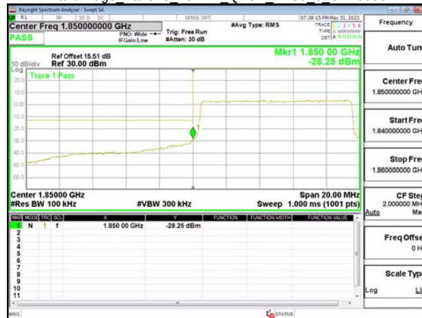
Band Edge Band25 10MHz QPSK RB50 0 CH26640
