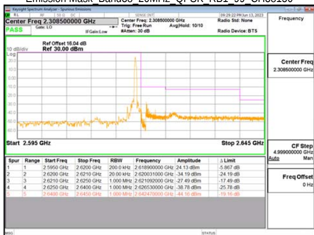
Emission Mask Band38 20MHz QPSK RB1 99 CH38150
