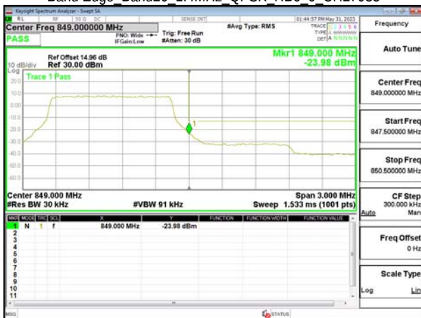
Band Edge Band26 1.4MHz QPSK RB6 0 CH27033
