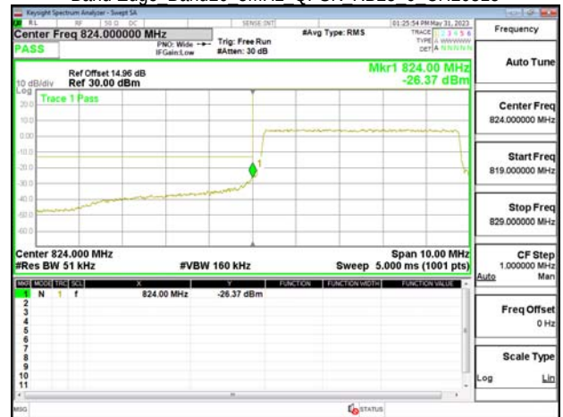
Band Edge Band26 5MHz QPSK RB25 0 CH27015
