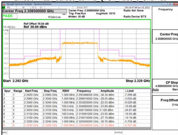
Emission Mask Band38 5MHz QPSK RB1 0 CH37775
