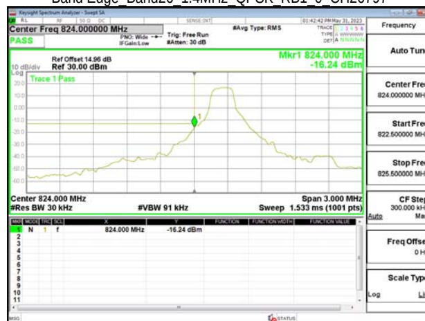
Band Edge Band26 1.4MHz QPSK RB1 0 CH26797
