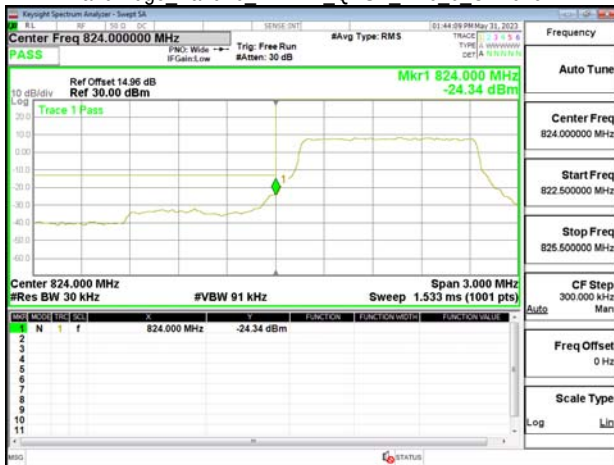
Band Edge Band26 1.4MHz QPSK RB6 0 CH27033
