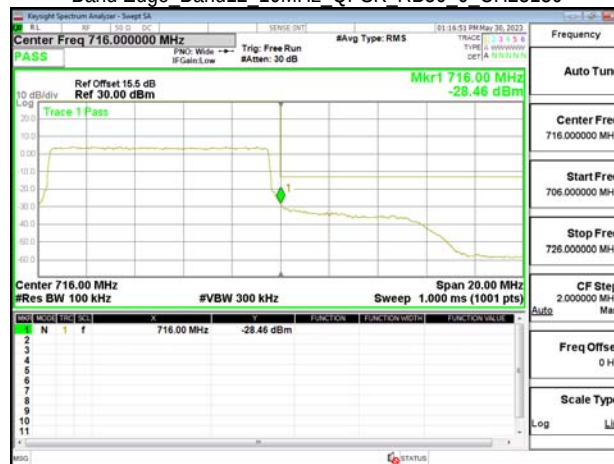
Band Edge Band12 10MHz QPSK RB50 0 CH23130
