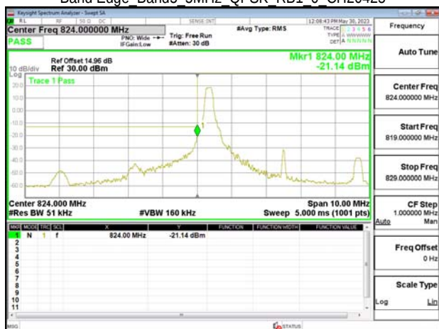
Band Edge Band5 5MHz QPSK RB1 0 CH20425
