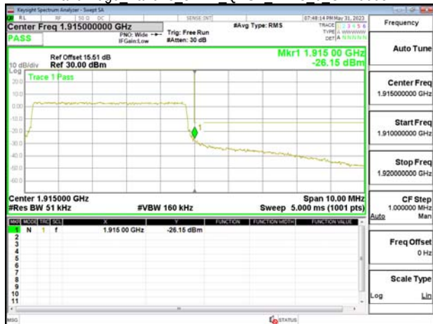
Band Edge Band25 10MHz QPSK RB1 0 CH26090
