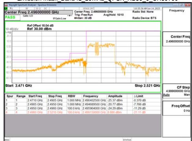
Emission Mask Band41 10MHz QPSK RB50 0 CH39700
