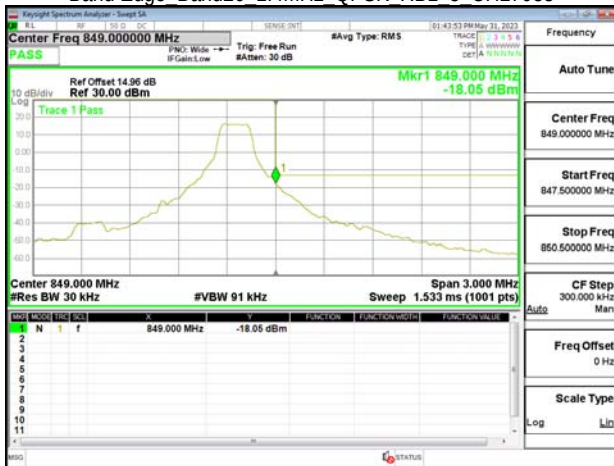
Band Edge Band26 1.4MHz QPSK RB6 0 CH26797
