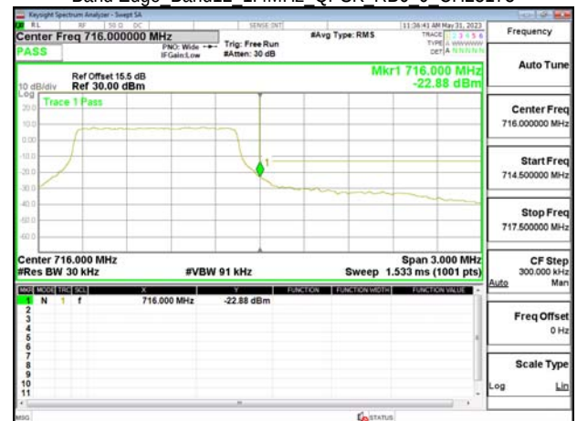
Band Edge Band12 1.4MHz QPSK RB6 0 CH23173
