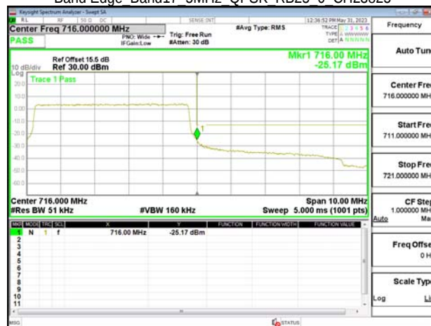
Band Edge Band17 10MHz QPSK RB1 0 CH23780
