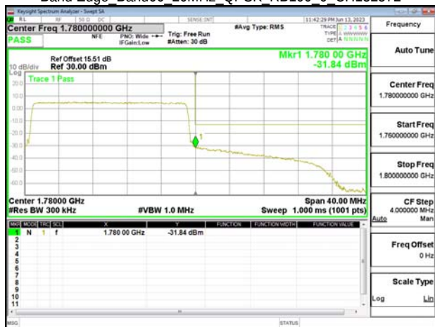
Band Edge Band66 20MHz QPSK RB100 0 CH132572
