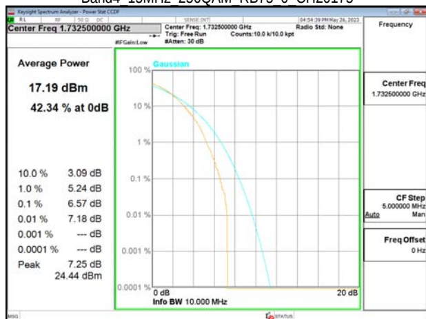
Band4 15MHz 256QAM RB75 0 CH20325
