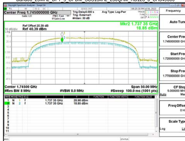
Band66 25MHz DFT s OFDM SCS15kHz 256QAM RB128 0 CH353500
