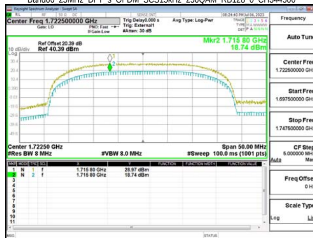
Band66 25MHz DFT s OFDM SCS15kHz 256QAM RB128 0 CH349000
