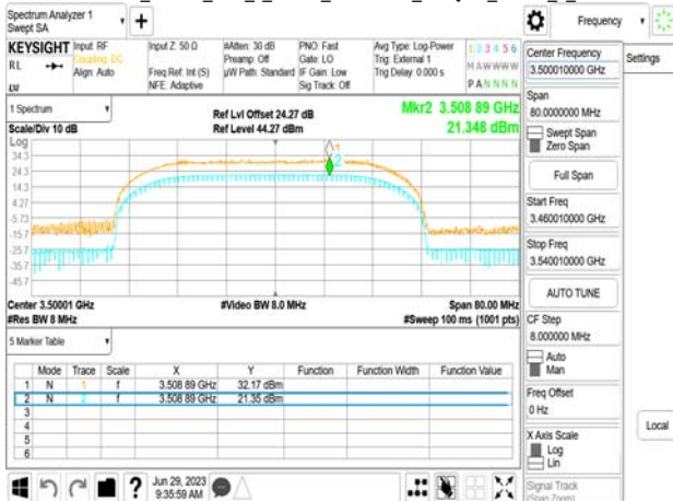
Band77-Part27 40MHz DFT_s_OFDM_SCS30kHz_256QAM_RB100_0_CH635332
