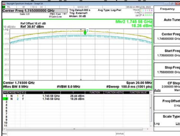
Band66 10MHz DFT s OFDM SCS15kHz 256QAM RB50 0 CH355000
