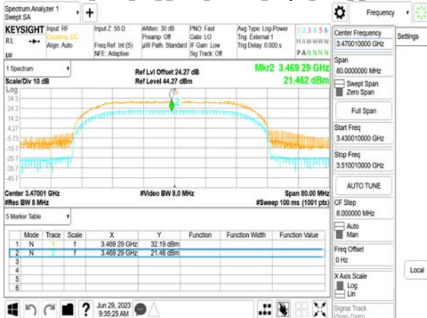
Band77-Part27 40MHz DFT_s_OFDM_SCS30kHz_256QAM_RB100_0_CH633334
