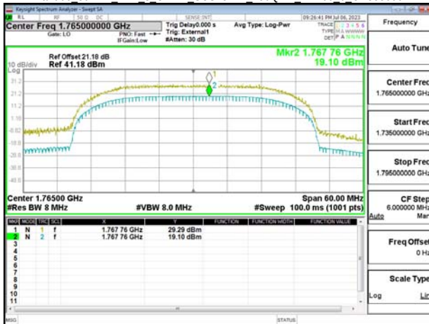
Band66 30MHz DFT s OFDM SCS15kHz 256QAM RB160 0 CH353000
