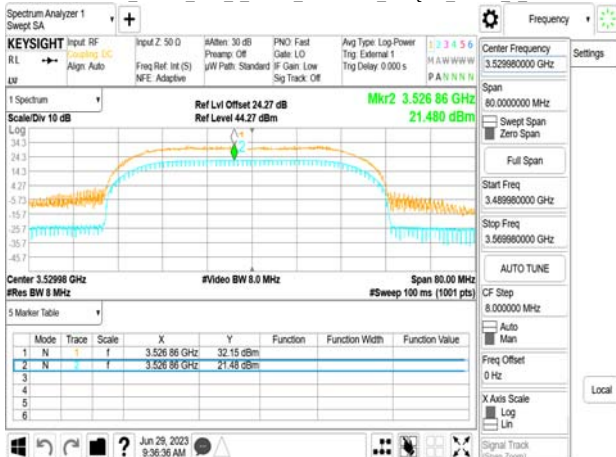
Band77-Part27 40MHz DFT_s_OFDM_SCS30kHz_256QAM_RB100_0_CH635332
