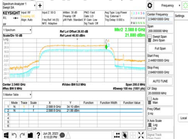
Band41 100MHz DFT s OFDM_SCS30kHz_256QAM_RB270_0_CH518598
