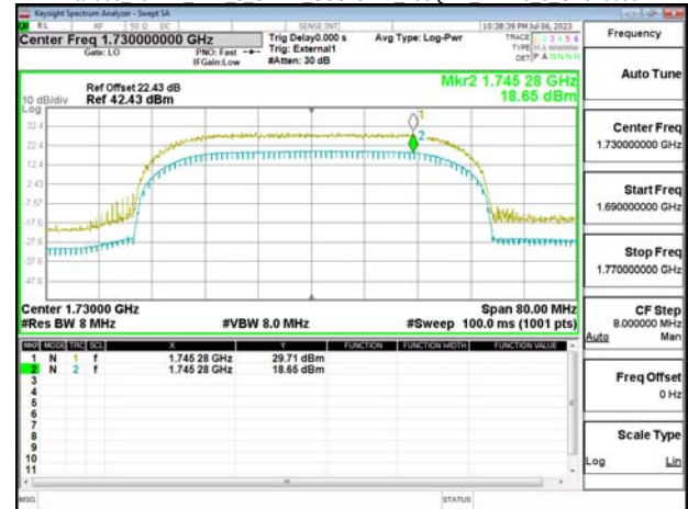
Band66 40MHz DFT s OFDM SCS15kHz 256QAM RB216 0 CH349000
