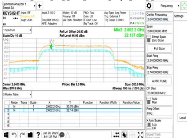
Band41 100MHz DFT s OFDM_SCS30kHz_256QAM_RB270_0_CH528000
