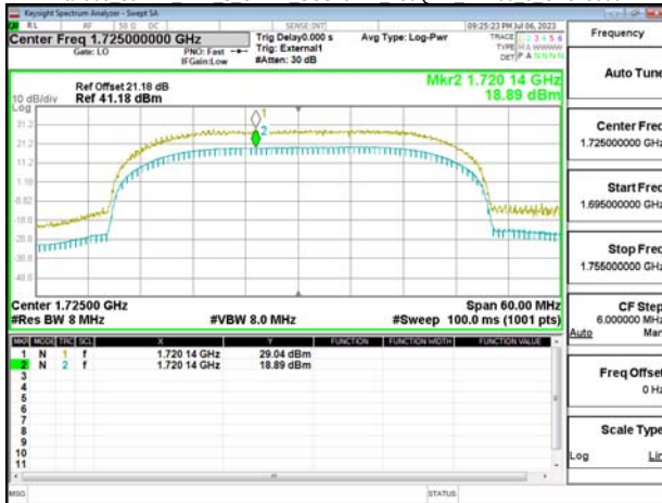
Band66 30MHz DFT s OFDM SCS15kHz 256QAM RB160 0 CH349000
