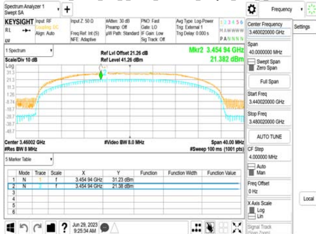
Band77-Part27_20MHz_DFT_s_OFDM_SCS30kHz_256QAM_RB50_0_CH633334
