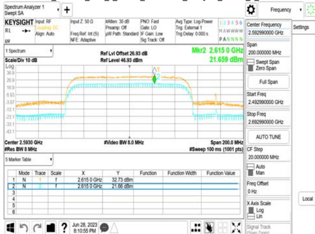
Band41 100MHz DFT s OFDM_SCS30kHz_256QAM_RB270_0_CH528000
