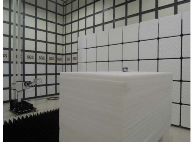
FCC 22 24 27 2 3G Radiated Setup
