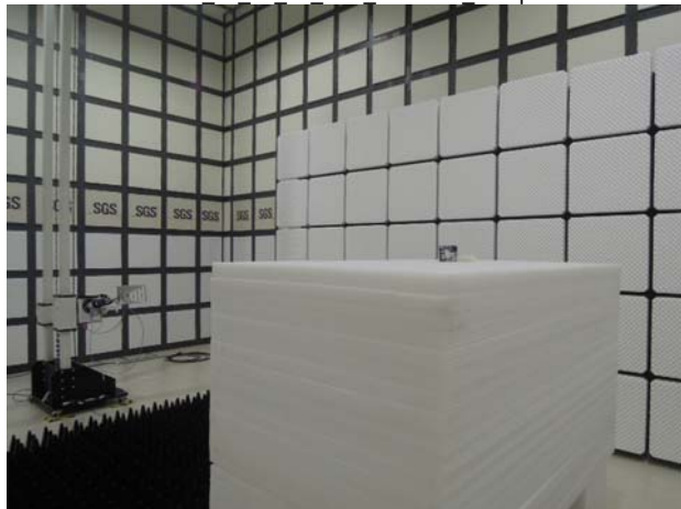
FCC 22 24 27 FR1 Radiated Setup
