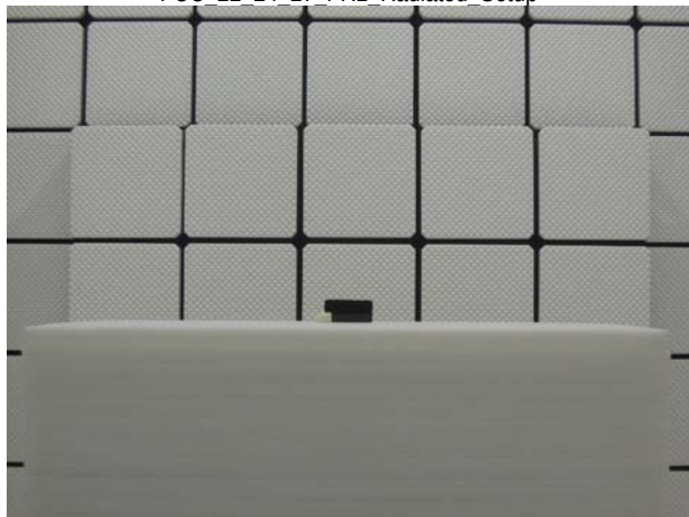
FCC 22 24 27 FR1 Radiated Setup
