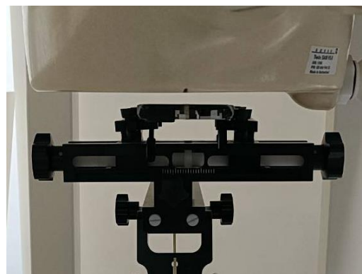
Photograph 10. Body-worn, Front Surface, 15mm
