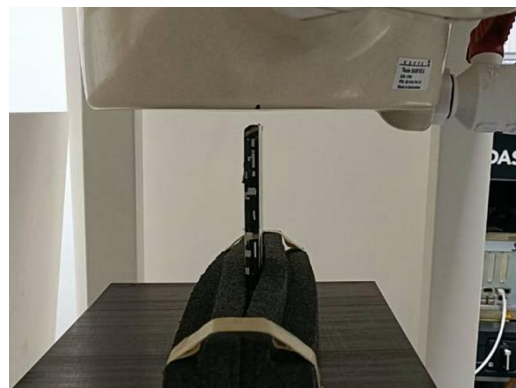
Photograph 20. Hotspot, Bottom Edge, 10mm
