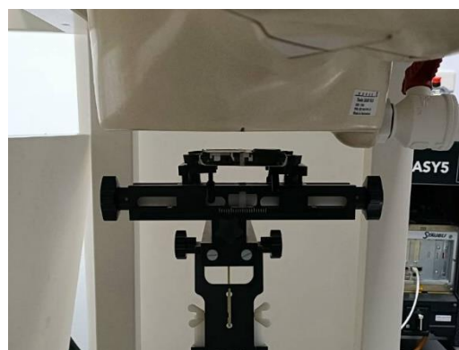
Photograph 12. Body-worn, Back Surface, 15mm
