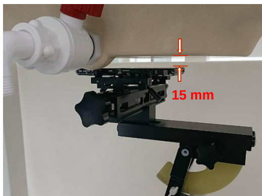
Photograph 9. Body-worn, Front Surface, 15mm
