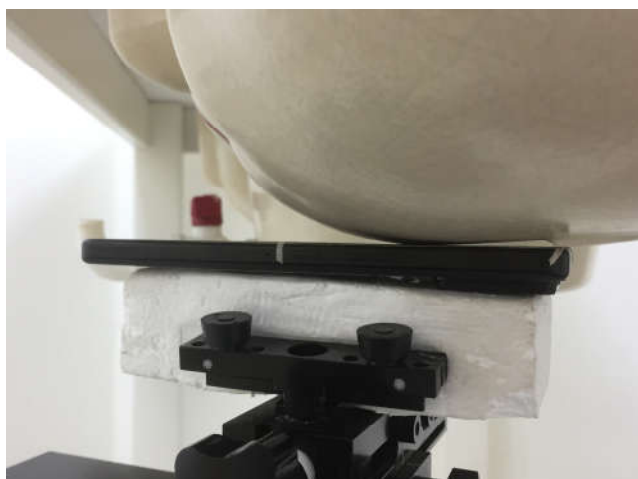
Left Cheek, Test Separation 0 mm
