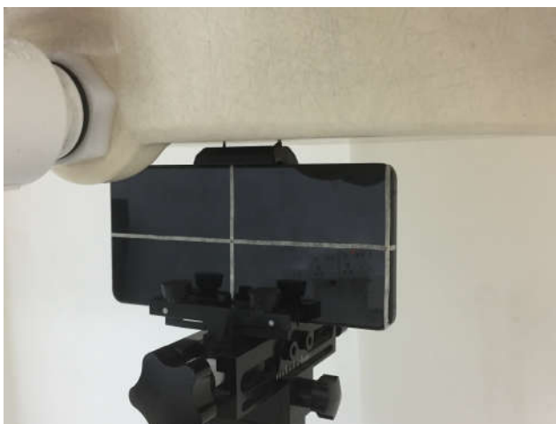
Left Side with AeroActive cooler, Test Separation 0 mm
