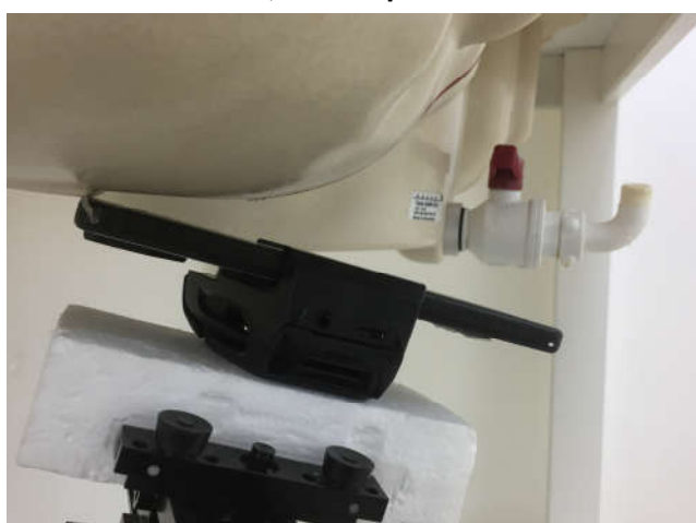
Right Tilted with AeroActive cooler, Test Separation 0 mm
