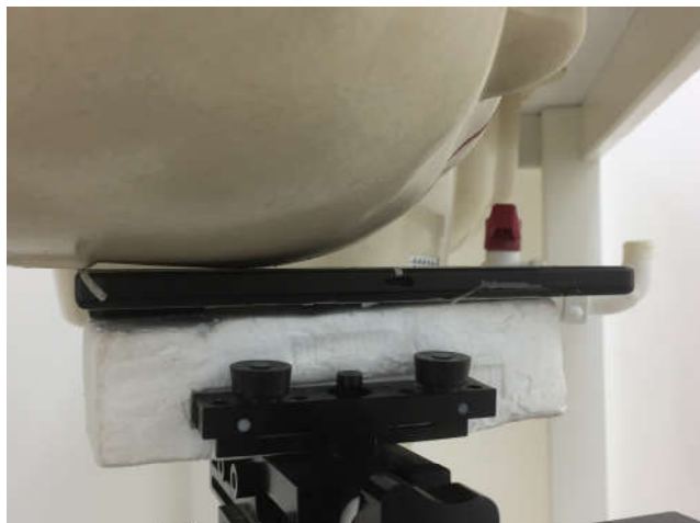
Right Cheek, Test Separation 0 mm
