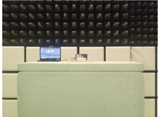
FCC 15 407 WLAN 6E Radiated Setup
