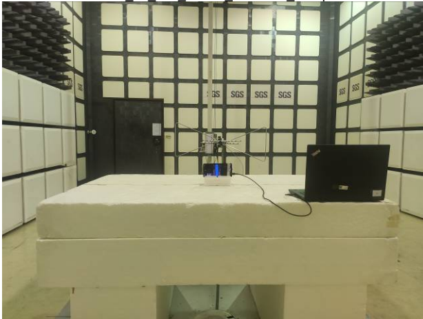
FCC 15 407 WLAN Radiated Setup
