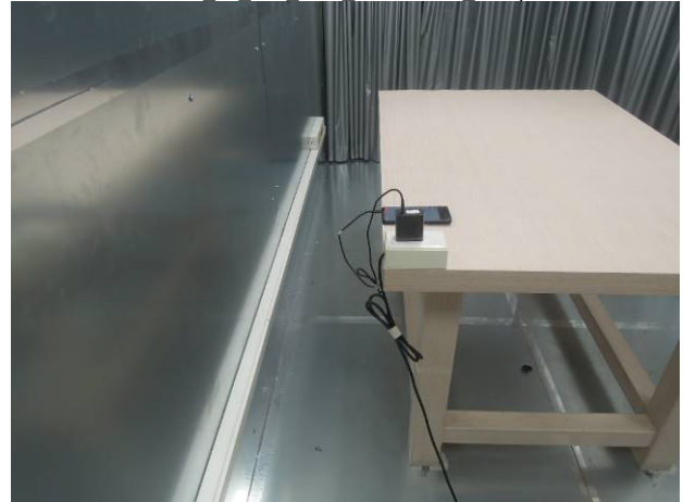
FCC 15 247 BLE Conduction Setup
