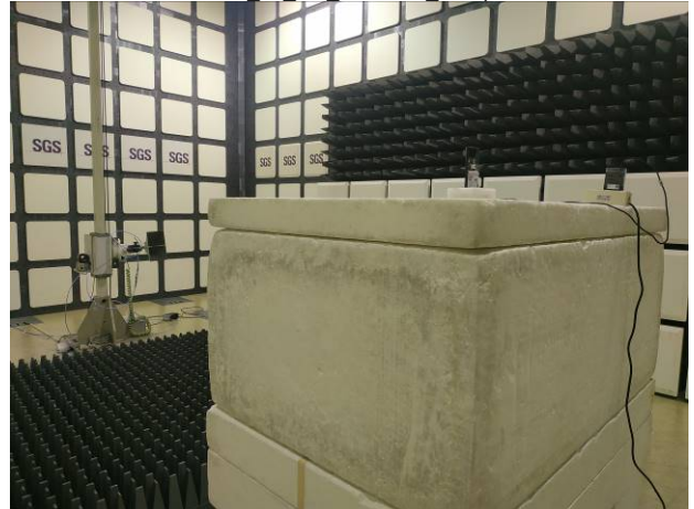
FCC 96 NR Radiated Setup
