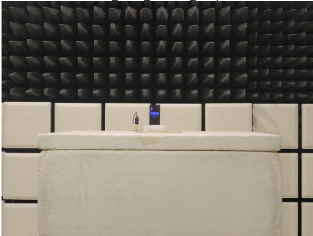
LTE ULCA Radiated Setup
