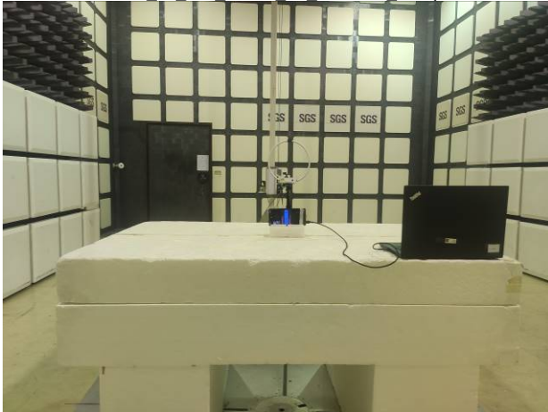
2 3G Radiated Setup
