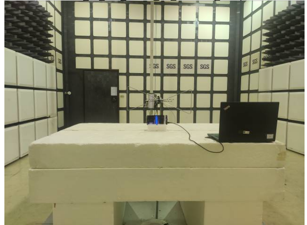
FCC 15 407 WLAN 6E Radiated Setup
