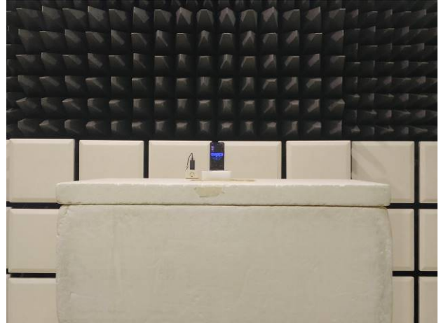
FCC 96 NR Radiated Setup
