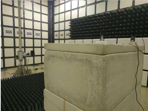
2 3G Radiated Setup
