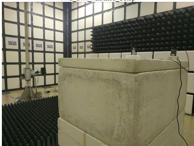
FR1 2TX Radiated Setup
