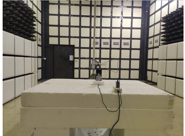
FCC 96 LTE Radiated Setup
