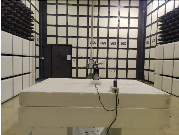
LTE ULCA Radiated Setup
