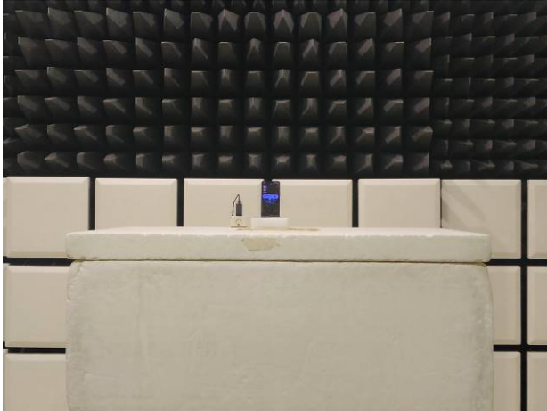
FCC 96 LTE ULCA Radiated Setup
