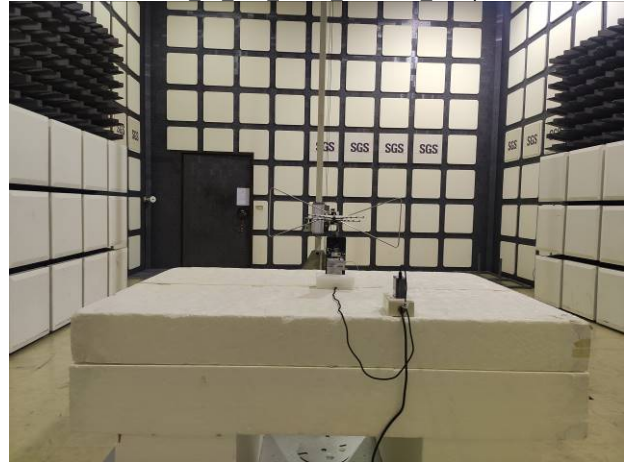
FCC 96 NR Radiated Setup
