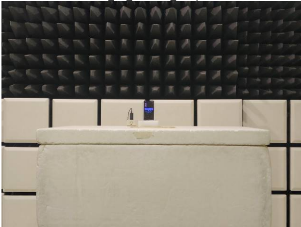
2 3G Radiated Setup
