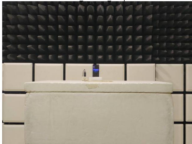
LTE Radiated Setup
