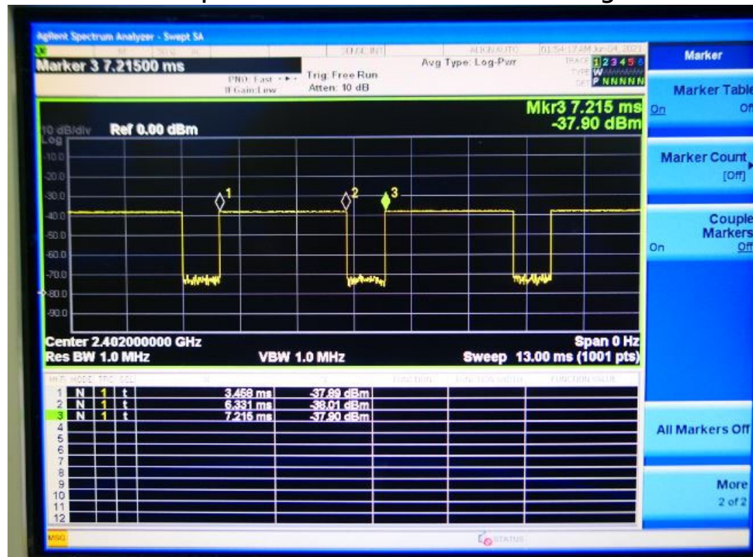
Time-domain plot for Bluetooth transmission signal
