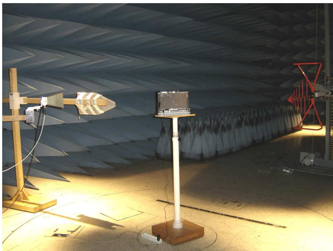
**TEST SET-UP FOR RADIATED MEASUREMENTS BELOW 1 GHz**
