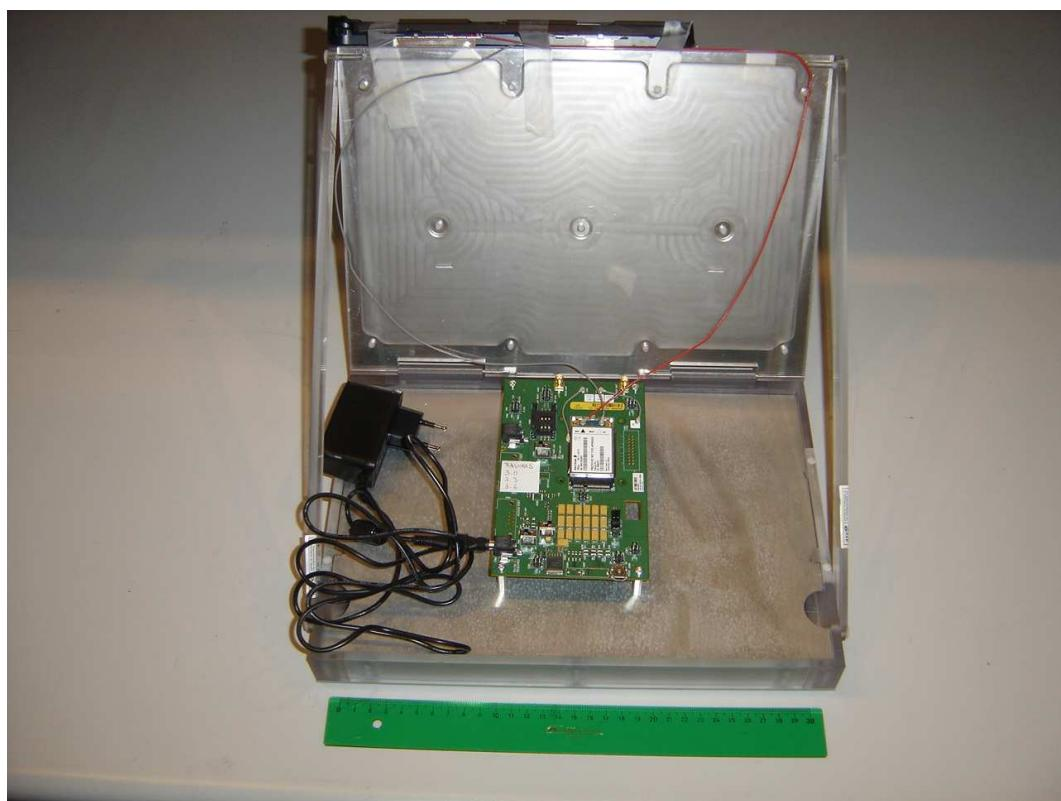
**GENERAL SET-UP FOR RADIATED MEASUREMENTS**
