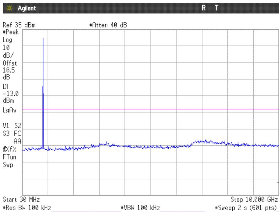
Note: The peak above the limit is the carrier frequency.
