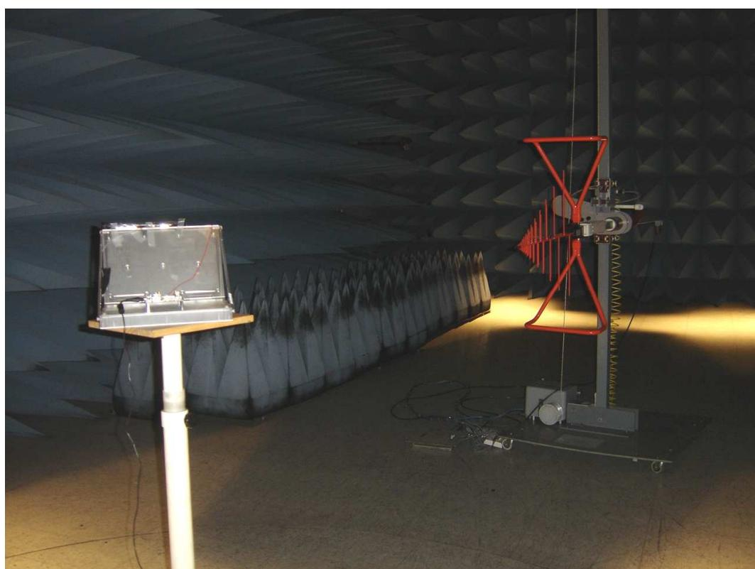
**TEST SET-UP FOR RADIATED MEASUREMENTS ABOVE 1GHz**
