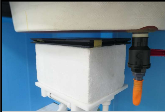
Rear Face of Tablet Mode Tested at 23 mm
