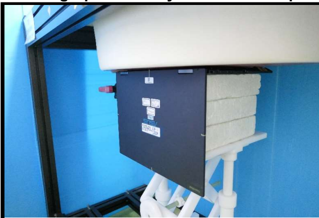
Bottom of Laptop Mode Tested at 0 mm
