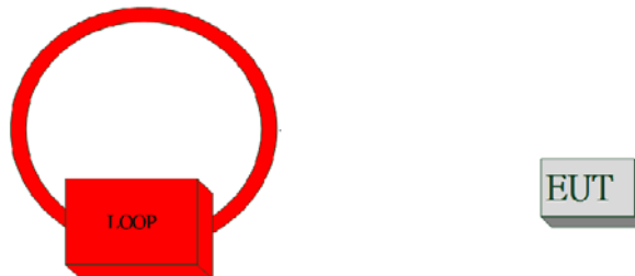
Fig. 2-2 Conduction test set up configuration
