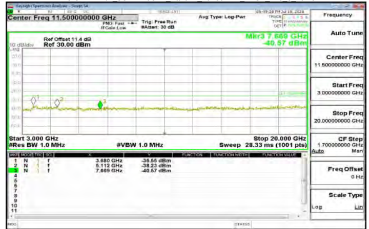
DFT-s-OFDM Pi/2 3GHz-26GHz Band41 20+80MHz BPSK 216 0 MidCH
