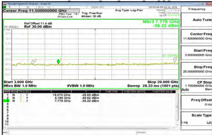
DFT-s-OFDM Pi/2 3GHz-26GHz Band41 20+80MHz BPSK 1 0 HighCH
