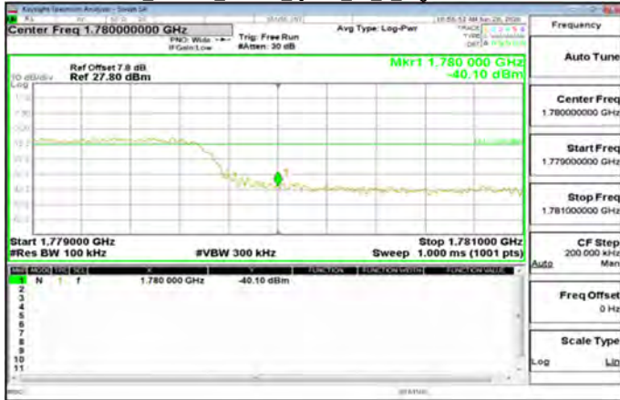
CP-OFDM Band66_15MHz_QPSK_1_0 LowCH343500-1717.5
