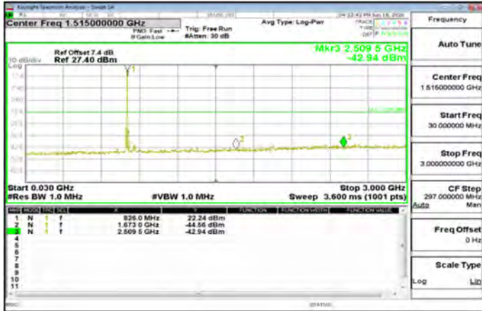
DFT-s-OFDM Pi/2 30MHz~3GHz_Band5 20MHz_BPSK 1_0 MidCH167300-836.5
