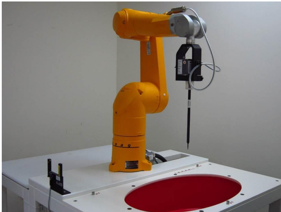
Fig.1 Photograph of the SAR measurement system
