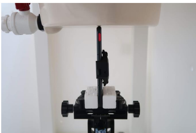
Bottom Side, Test Separation 0 mm _ AeroActive cooler
