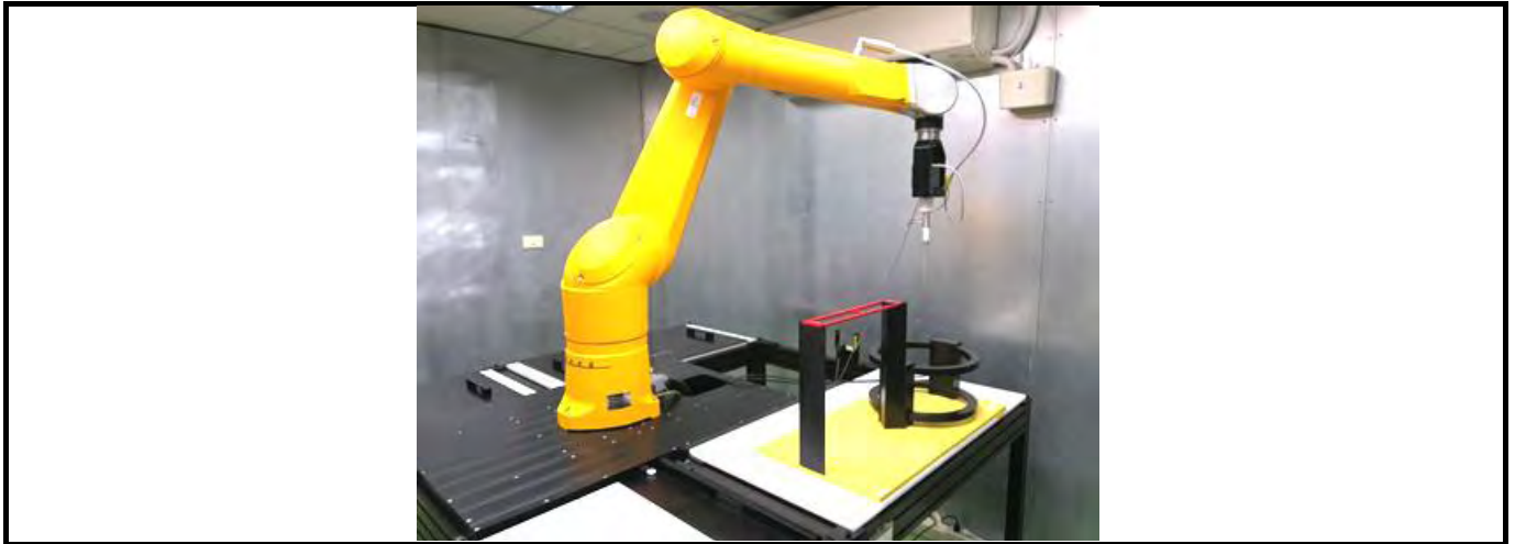
Fig-3.3 DASY52 Measurement System
