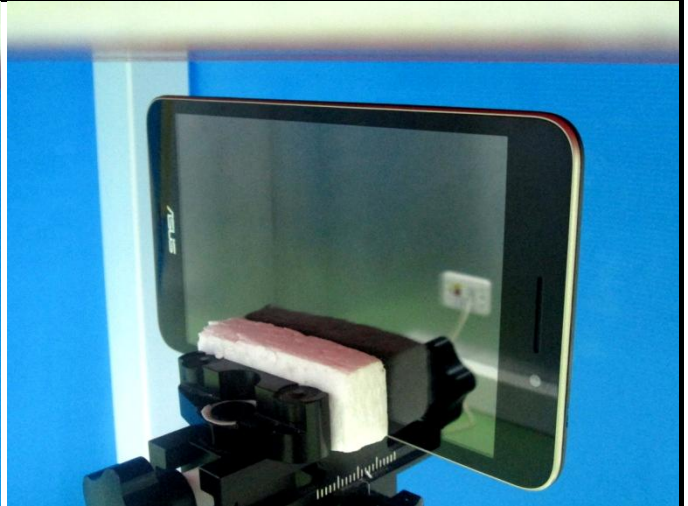
Left Side of EUT with 1.5 cm Gap
