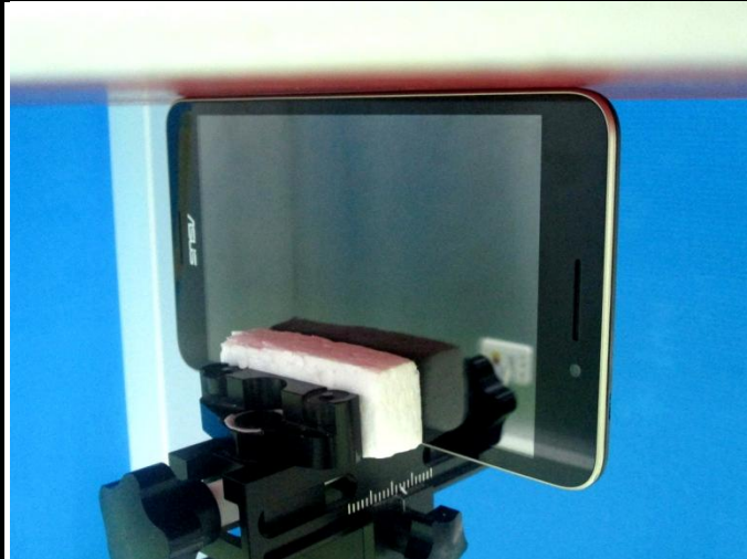
Left Side of EUT with 0 cm Gap
