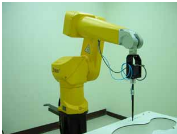
Fig. 5.2 Probe setup on robot
