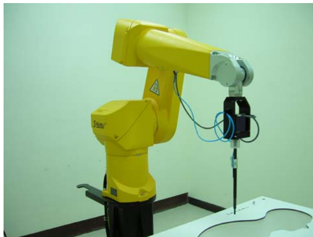
Fig. 5.2 Probe setup on robot
