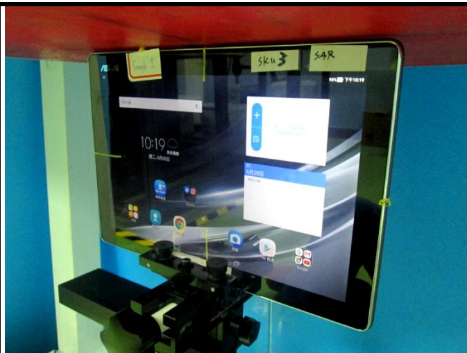
Body - Top Side of EUT 1 at 0 mm
