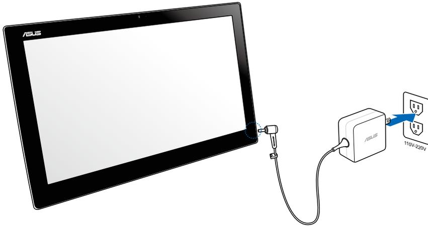
Connect the power adapter to your ASUS Portable AiO's DC-in port and plug to the correct socket outlet with the correct input rating. The input voltage of the adapter is 100Vac~240Vac.
