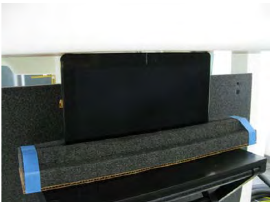
Fig.8 EUT Secondary Landscape mode to flat phantom (Test distance is 0 mm)
