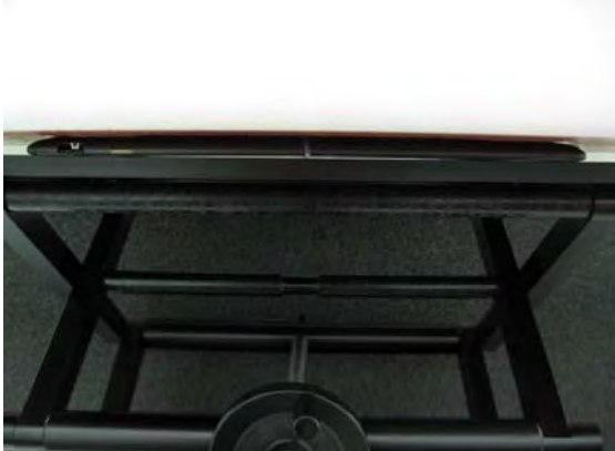
Fig.3 EUT Lap held mode to flat phantom (Test distance is 0 mm)
