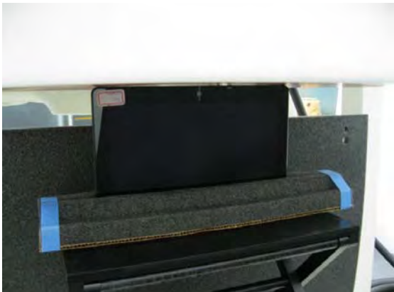
Fig.7 EUT Primary Landscape mode to flat phantom (Test distance is 0 mm)
