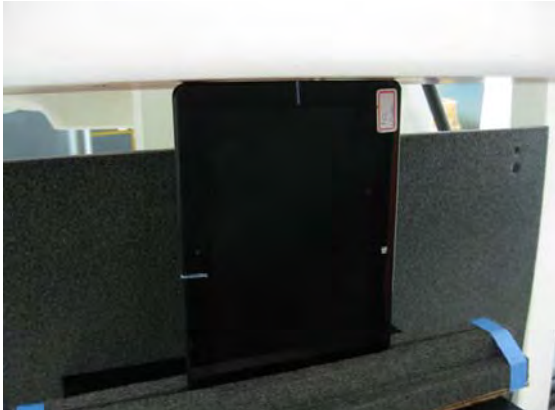
Fig.6 EUT Secondary Portrait mode to flat phantom (Test distance is 0 mm)
