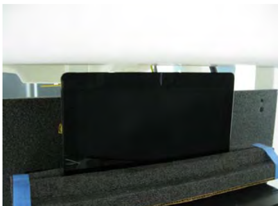
Fig.9 EUT Secondary Landscape mode to flat phantom (Test distance is 11 mm)
