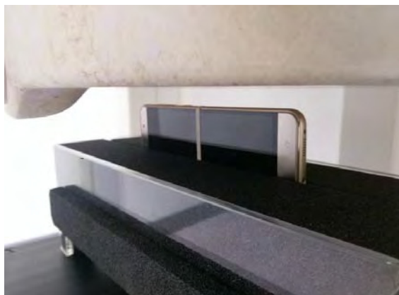
Fig.14 EUT Right side to flat phantom
