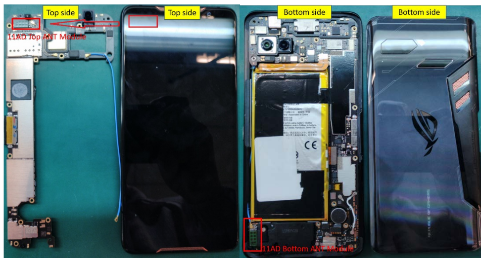
Figure C-1 802.11ad antenna module inside ASUS_Z01QD
