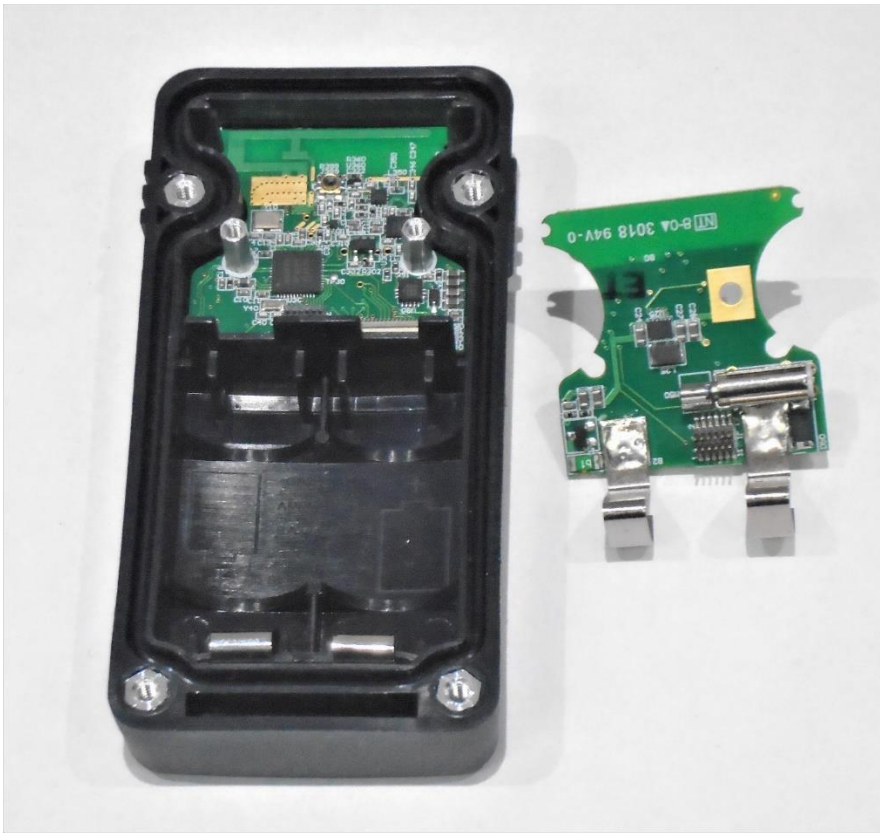
Interior with first PCB installed.
