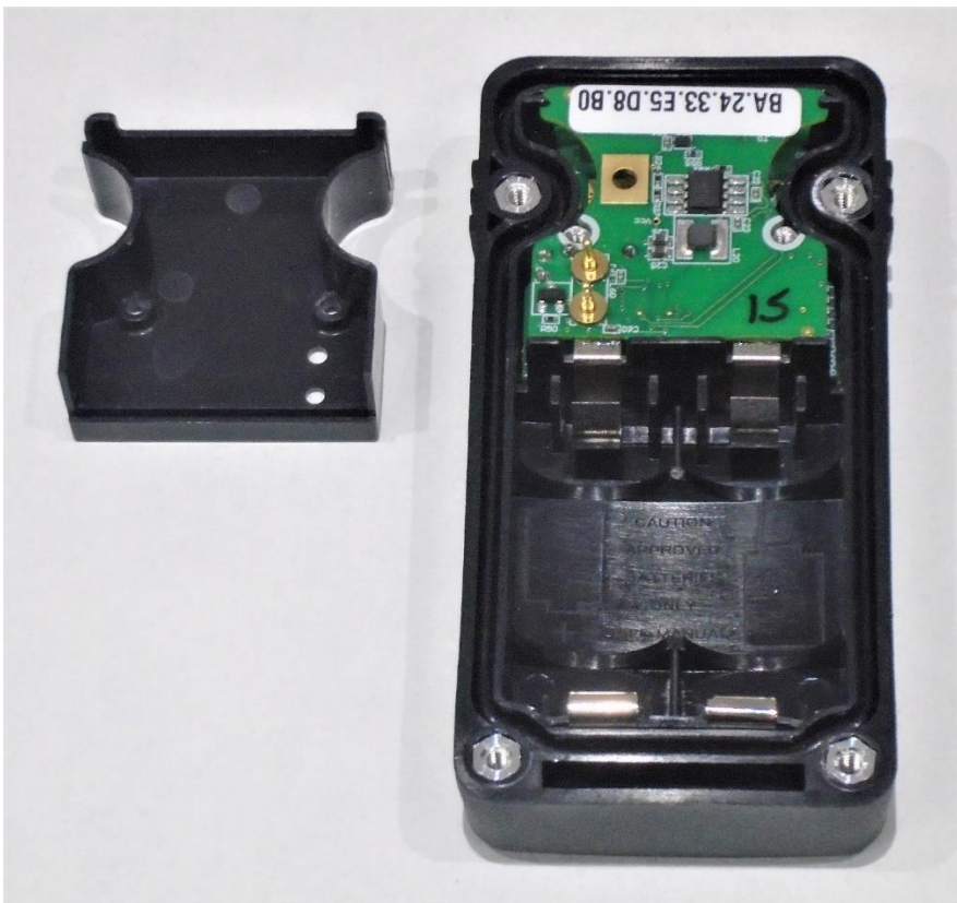
Interior with both PCBs Installed.
