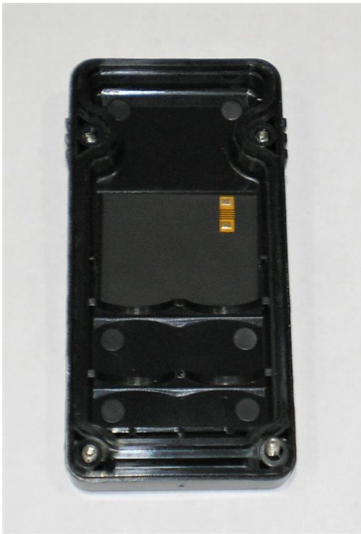
NFC antenna mounted in case back showing contacts and ferrite side.
