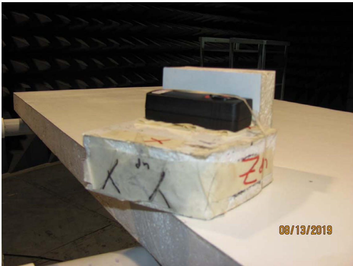
The EUT was taped to a foam stand to change the axis of rotation.
